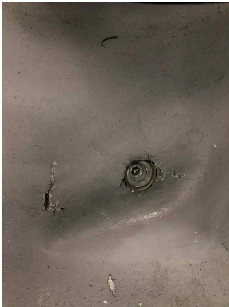
Photo 2 - View of damage to the monocoque cabin behind the right seat (Courtesy of FAA)
