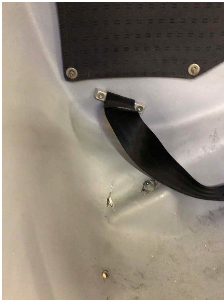
Photo 1 – View of damage to the monocoque cabin behind the right seat (Courtesy of FAA)
