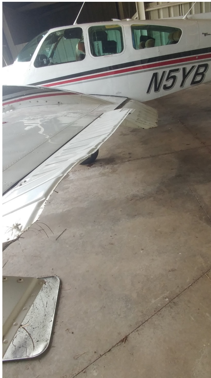
Photo 1 – View of damaged left aileron (Photo courtesy of the FAA)
