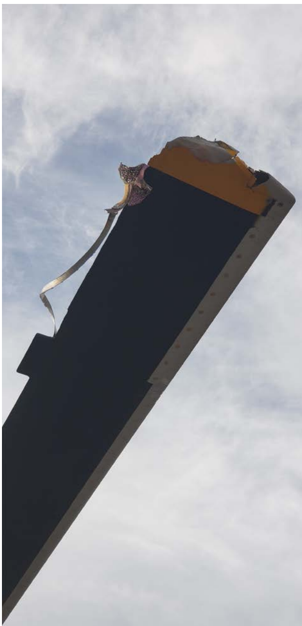
Photo 1 – View of damaged main rotor blade (courtesy of the operator)
