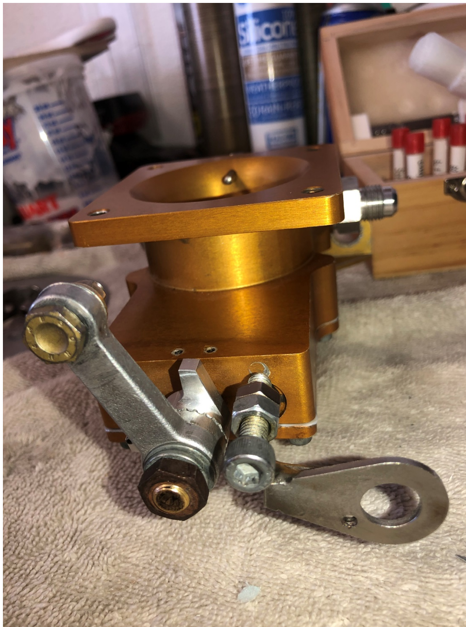
Photo 3 – View of bent idle stop screw on modified carburetor (Photo courtesy of the FAA)
