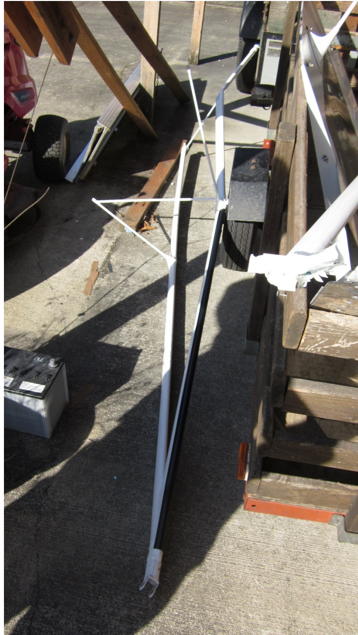
Photo 2 – View of damaged left wing lift strut (Photo courtesy of the FAA)
