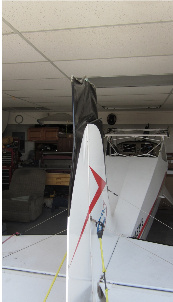
Photo 1 – View of damaged rudder (Photo courtesy of the FAA)
