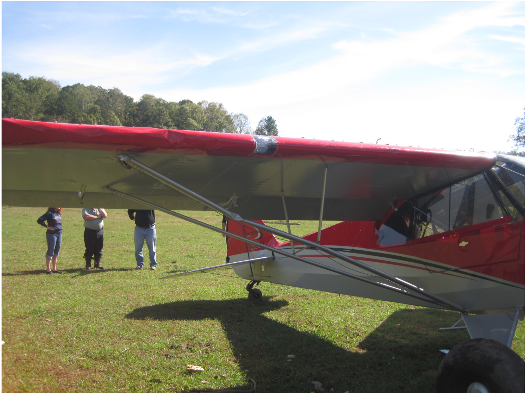
Photo 1 – View of damage to right wing lift strut (Courtesy of FAA)
