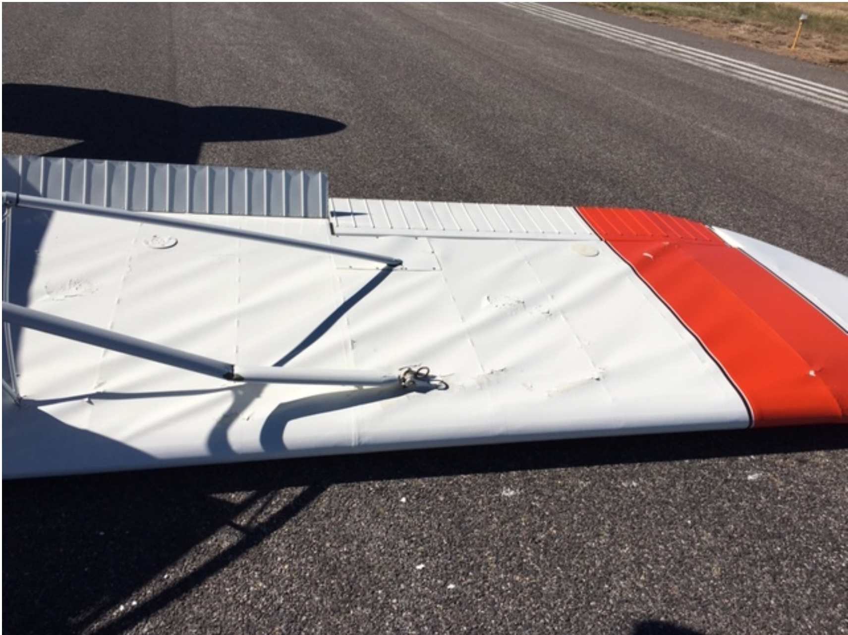
Photo 1 – View of damaged right wing lift strut (Photo courtesy of Airport Operations)
