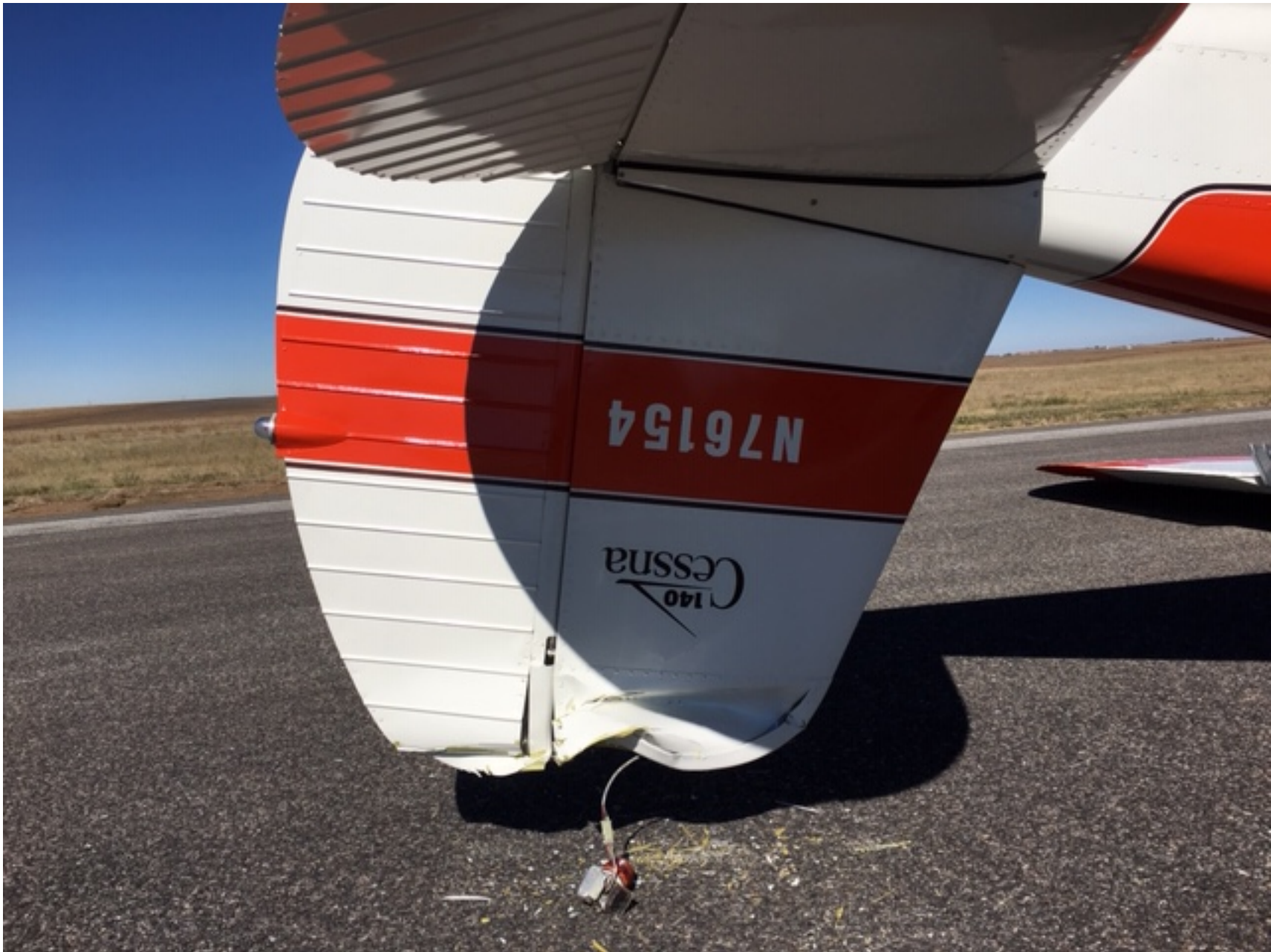
Photo 2 – View of damaged vertical stabilizer and rudder (Photo courtesy of Airport Operations)
