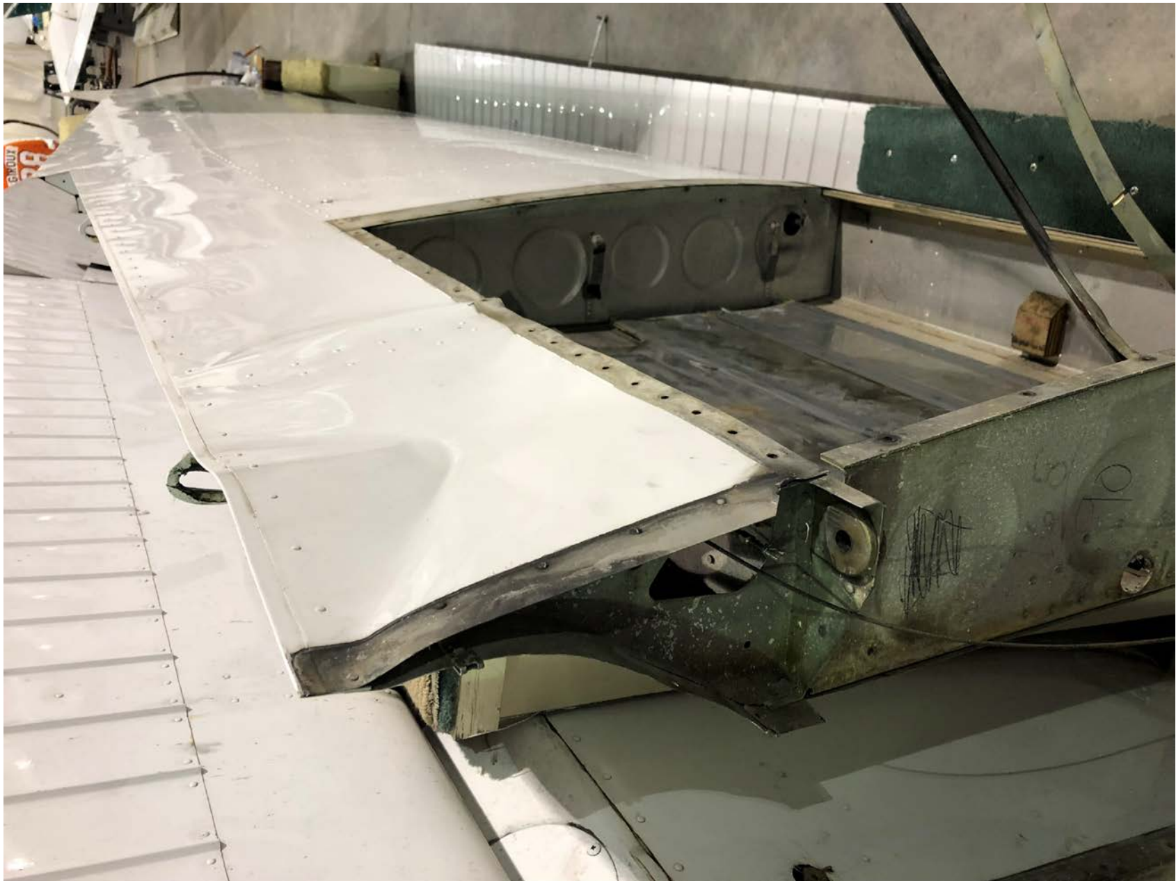
Photo 1 – View of damage to the left wing rear spar (Courtesy of FAA)
