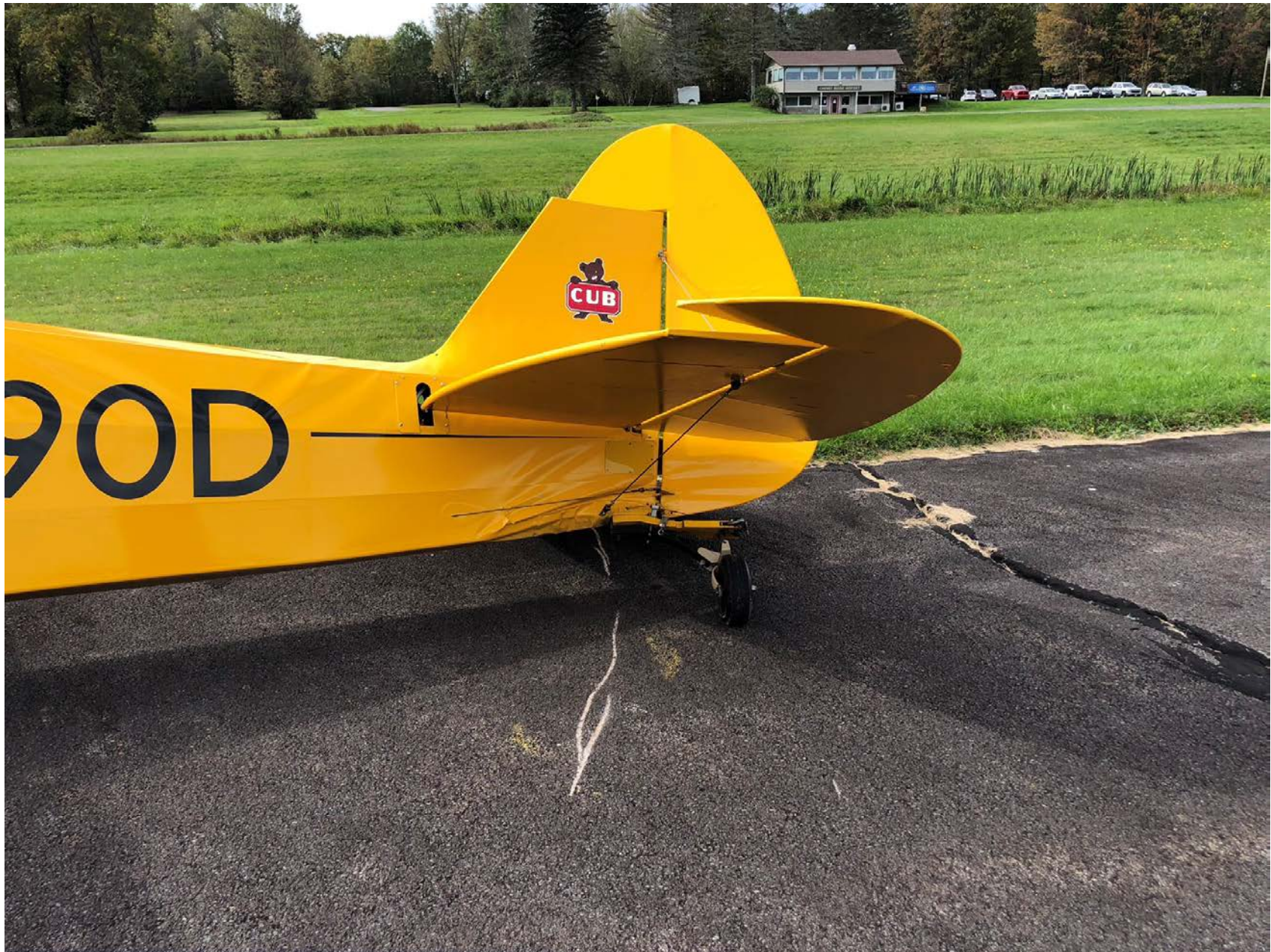
Photo 2 – View of damaged rudder (courtesy of the pilot)
