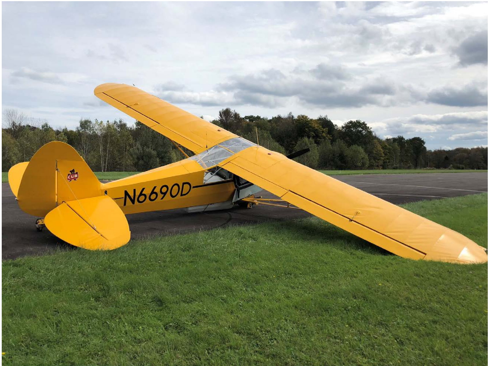
Photo 1 – View of damaged right wing (courtesy of the pilot)
