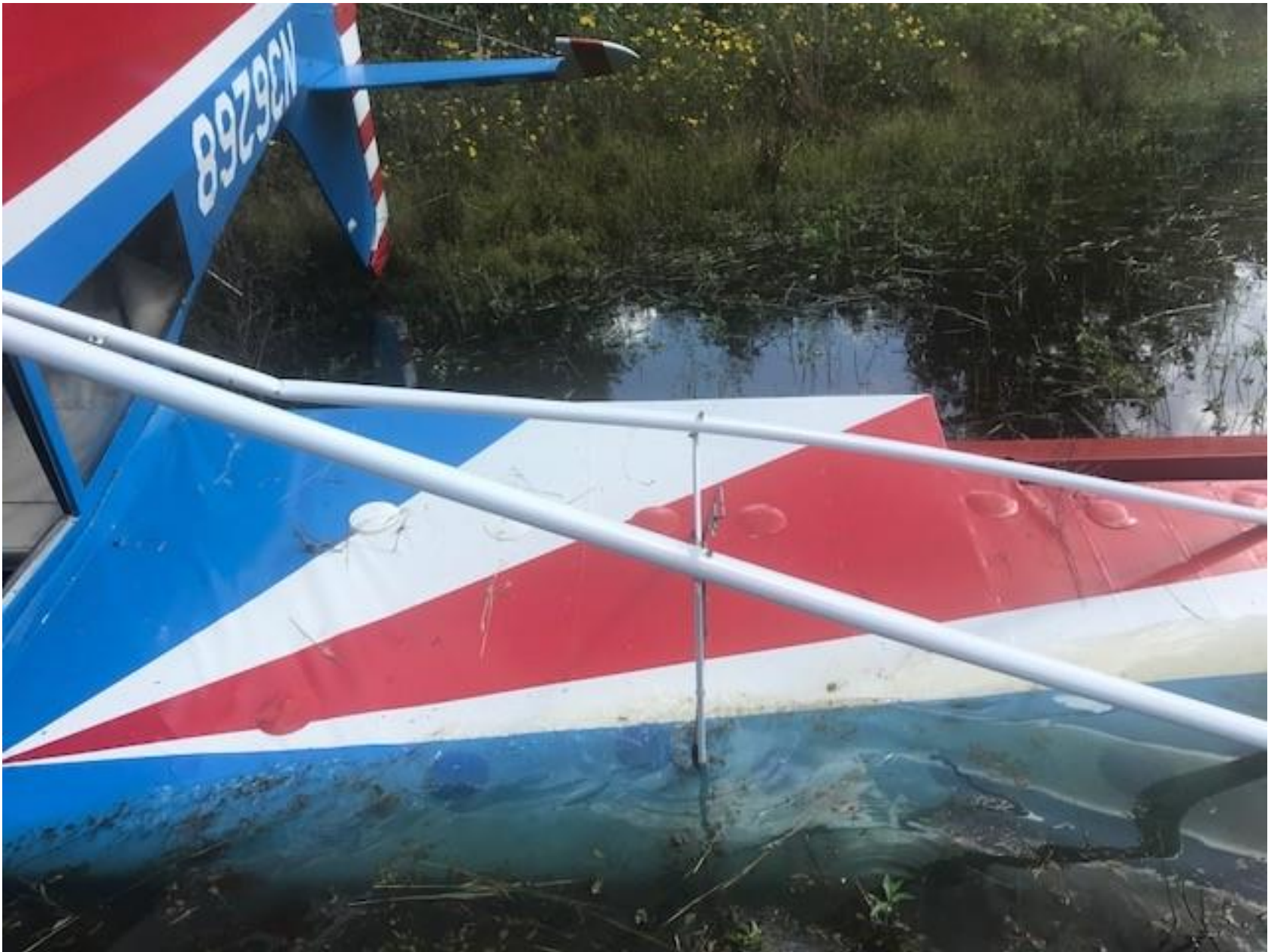
Photo 2 – View of damaged right wing lift strut (Photo courtesy of the FAA)
