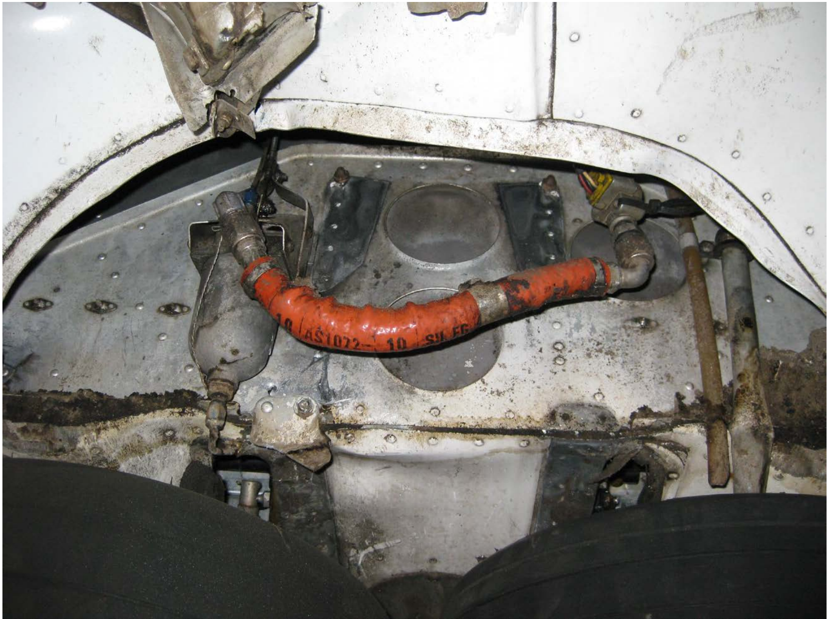
Photo – View of damage to tunnel structure and lower fuselage skin aft of firewall (courtesy of the FAA)
