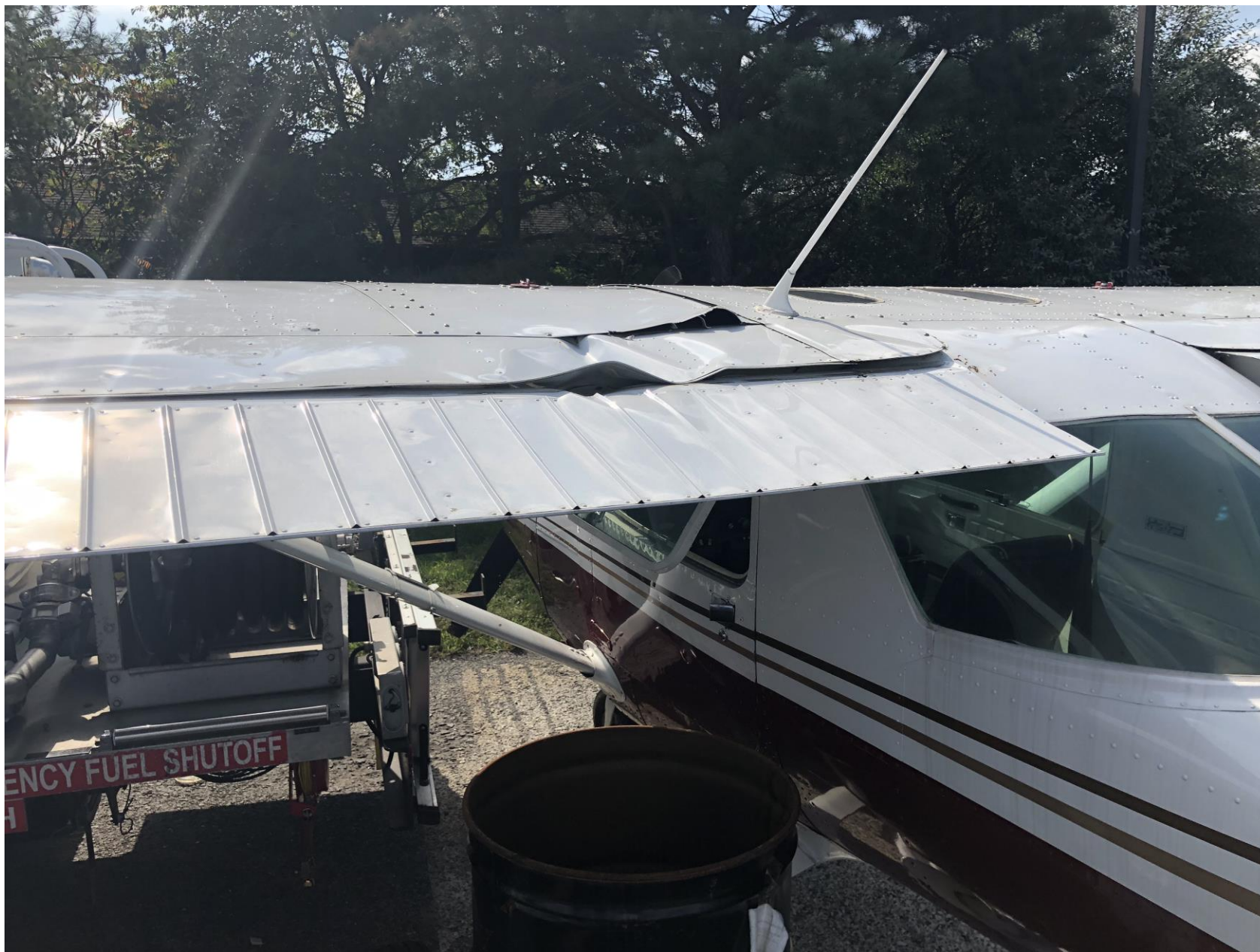
Photo 2 – Rear view of damaged left wing (Photo courtesy of the FAA)
