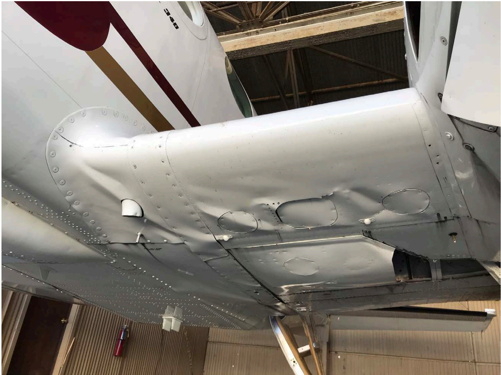
Photo 1 – View of damage to left wing (photo courtesy of the FAA)
