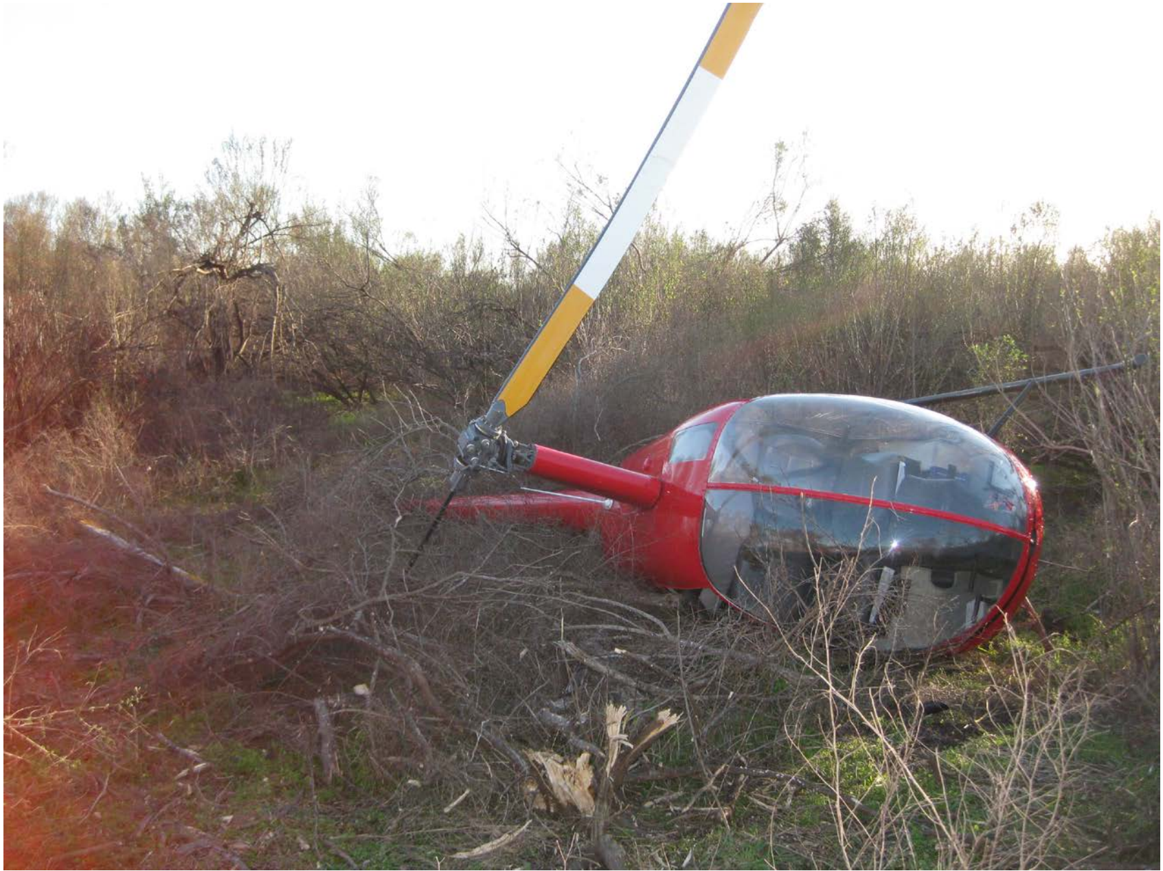
Photo 1 – View of damage to main rotor blades (Courtesy of FAA)
