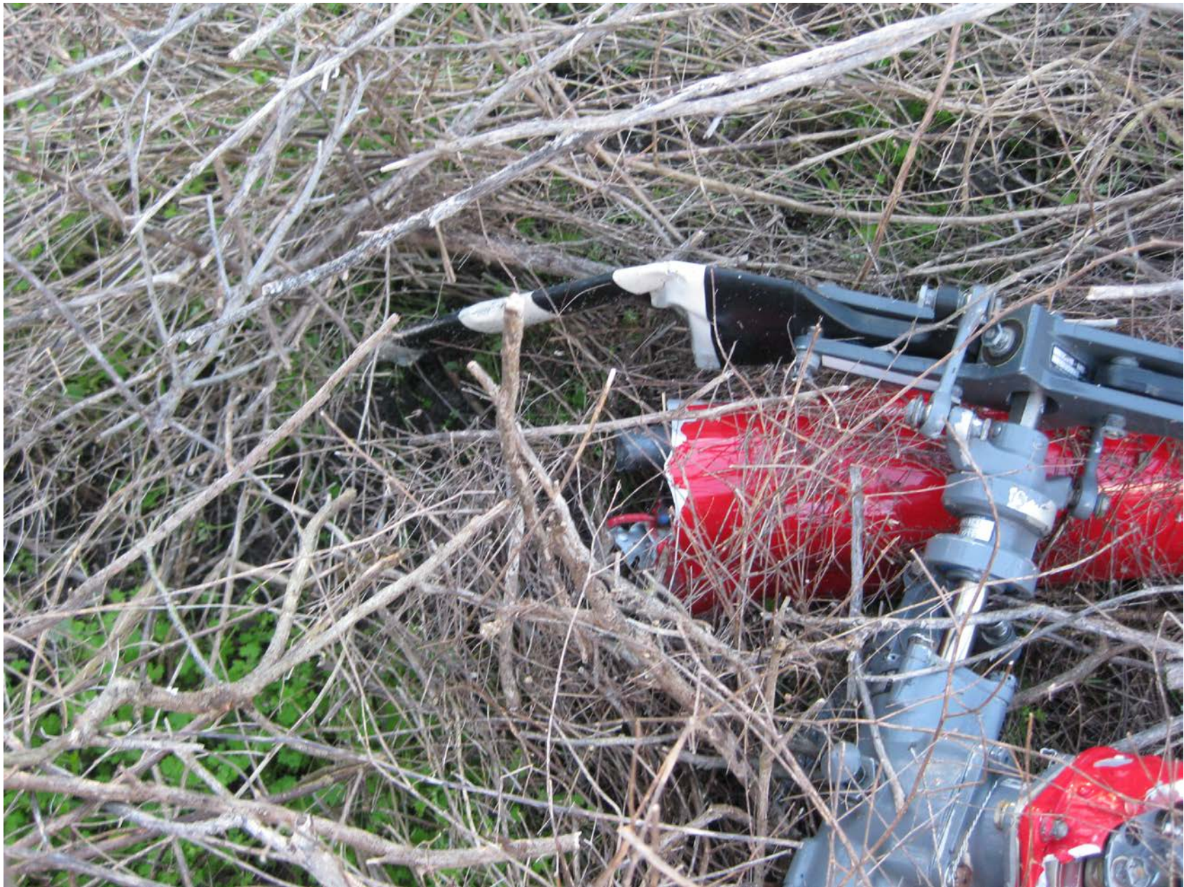
Photo 2 – View of damage to tail rotor drive system (Courtesy of FAA)
