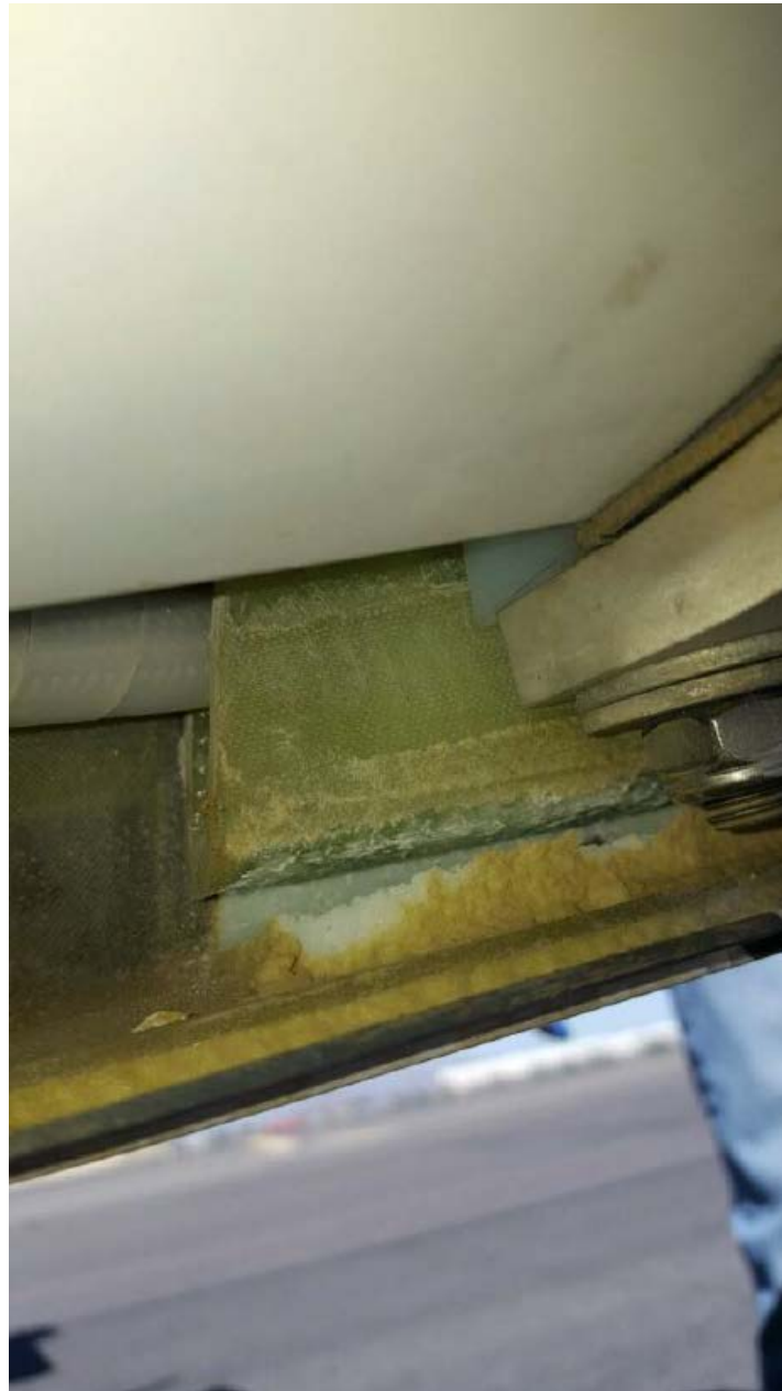
Photo 3 - View of damage to the right main landing gear attachment mount and airframe structure -Image was taken looking toward the tail of airplane (Courtesy of FAA)
