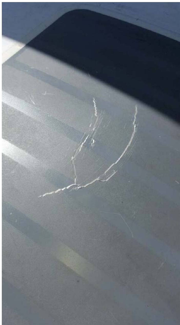
Photo 1 – View of damage to the wing walk (Courtesy of FAA)
