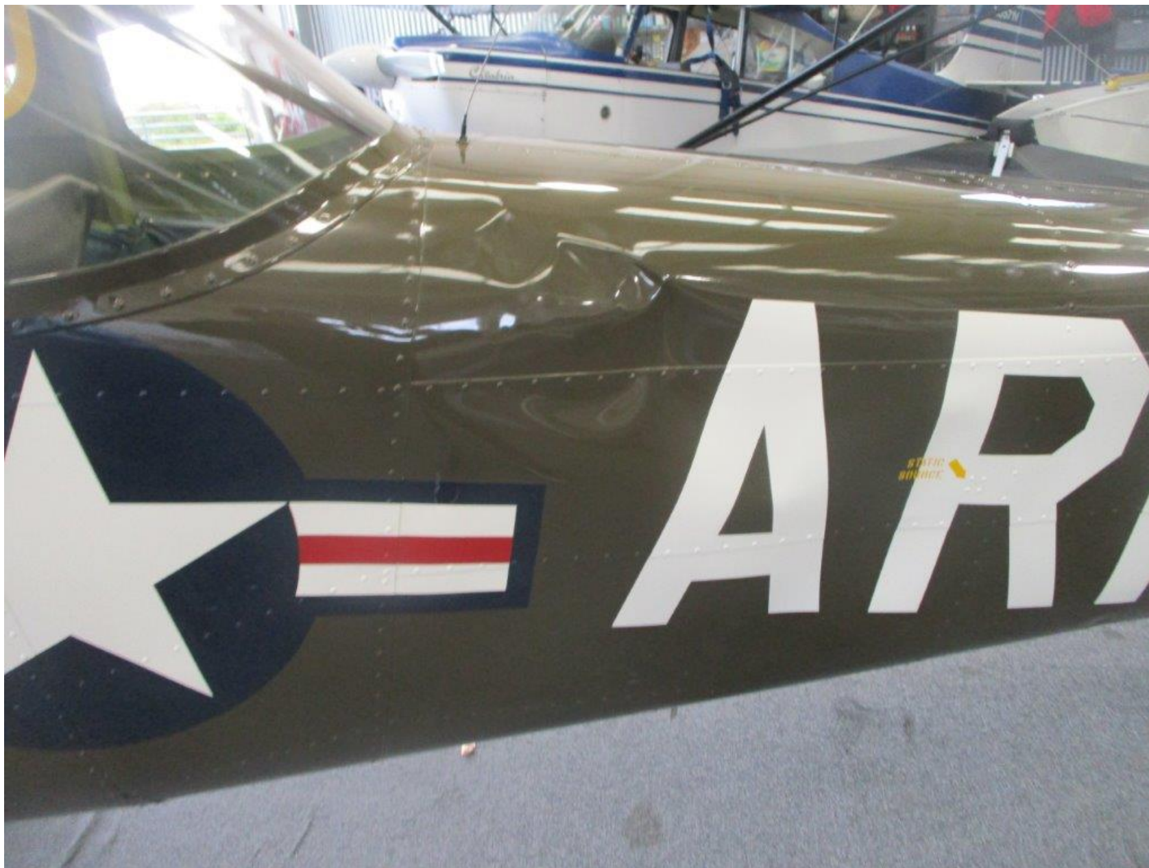
Photo 1 – View of damaged tailcone (courtesy of the repair station)
