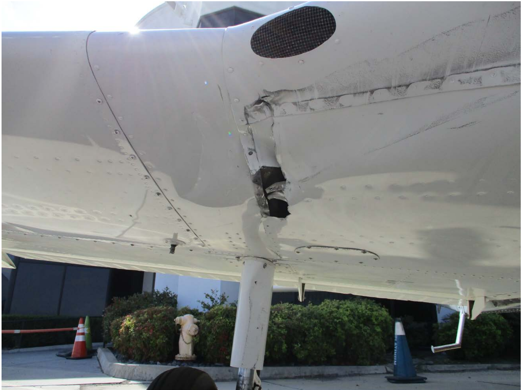
Photo 1 – View of damage to the bottom of the right wing (Courtesy of FAA)
