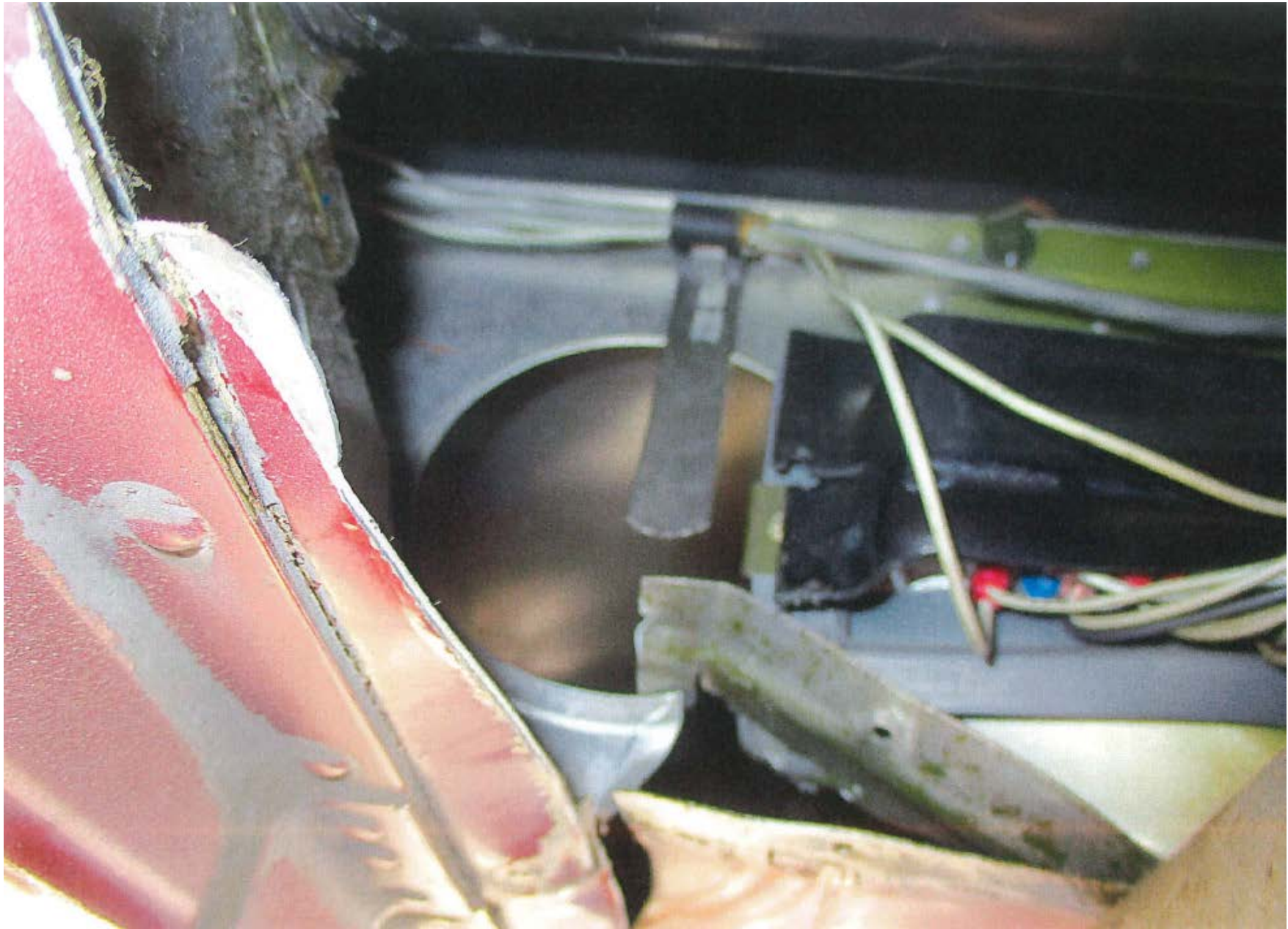
Photo 2 – View of damage to the lower fuselage intermediate bulkhead (Courtesy of Repair Station)
