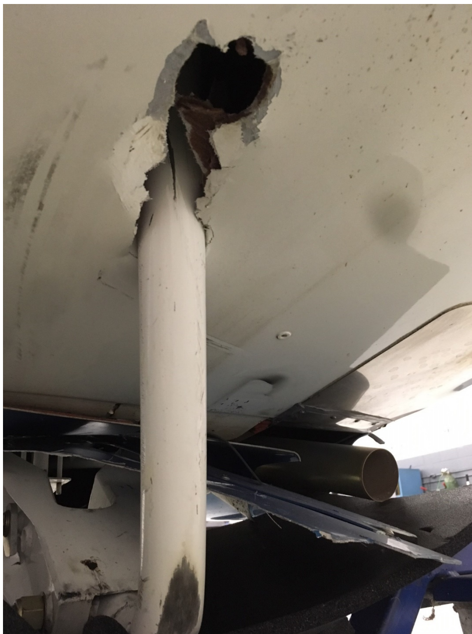
Photo 1 – View of damage to the forward lower fuselage (Courtesy of FAA)
