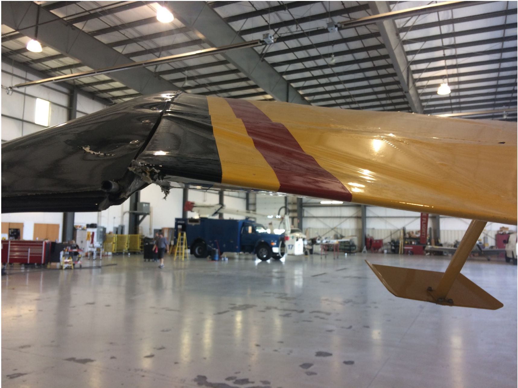
Photo 1 – View of damaged left aileron (Photo courtesy of the pilot)
