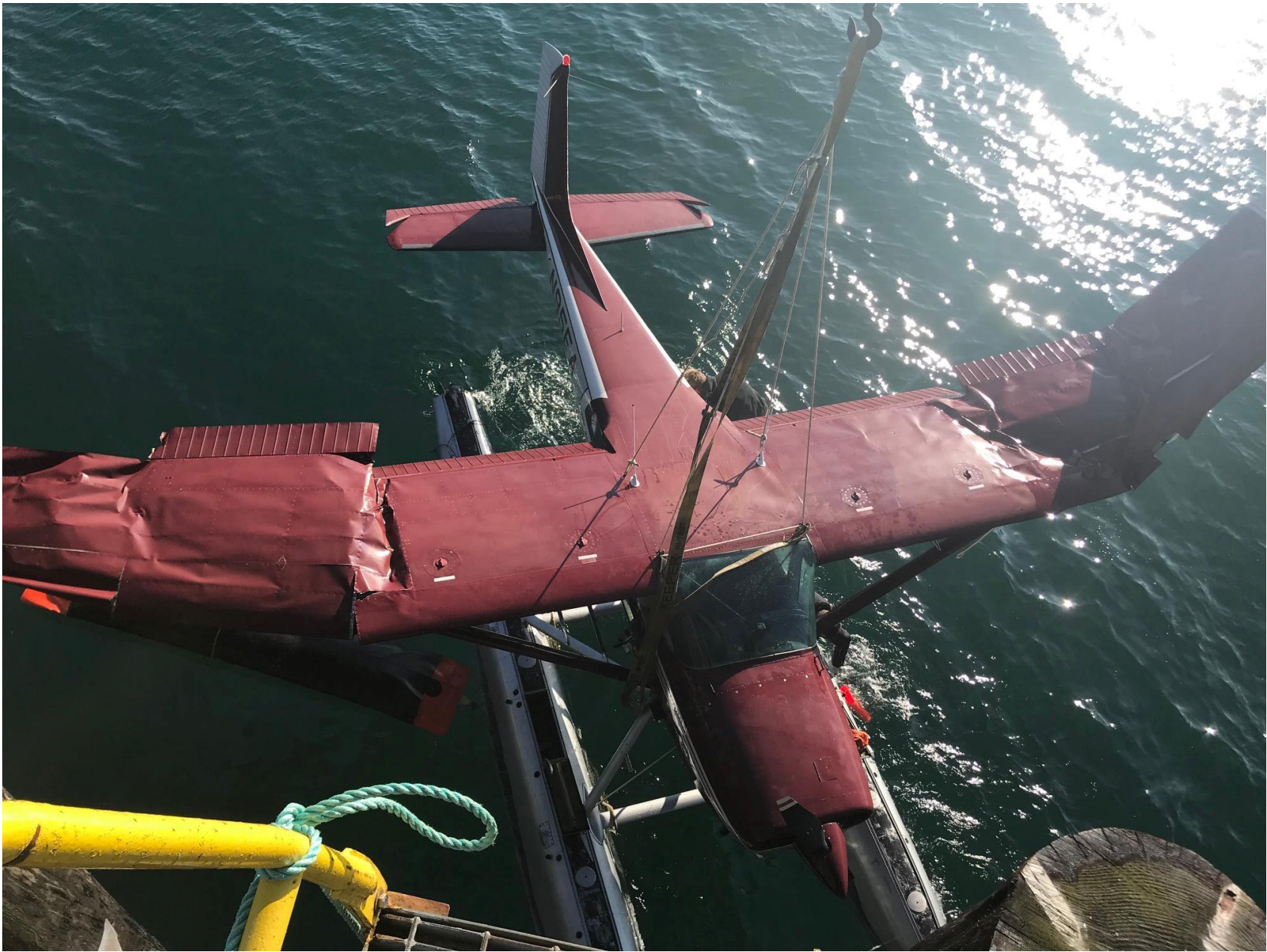
Photo 1 – View of damaged wings (Photo courtesy of the pilot)
