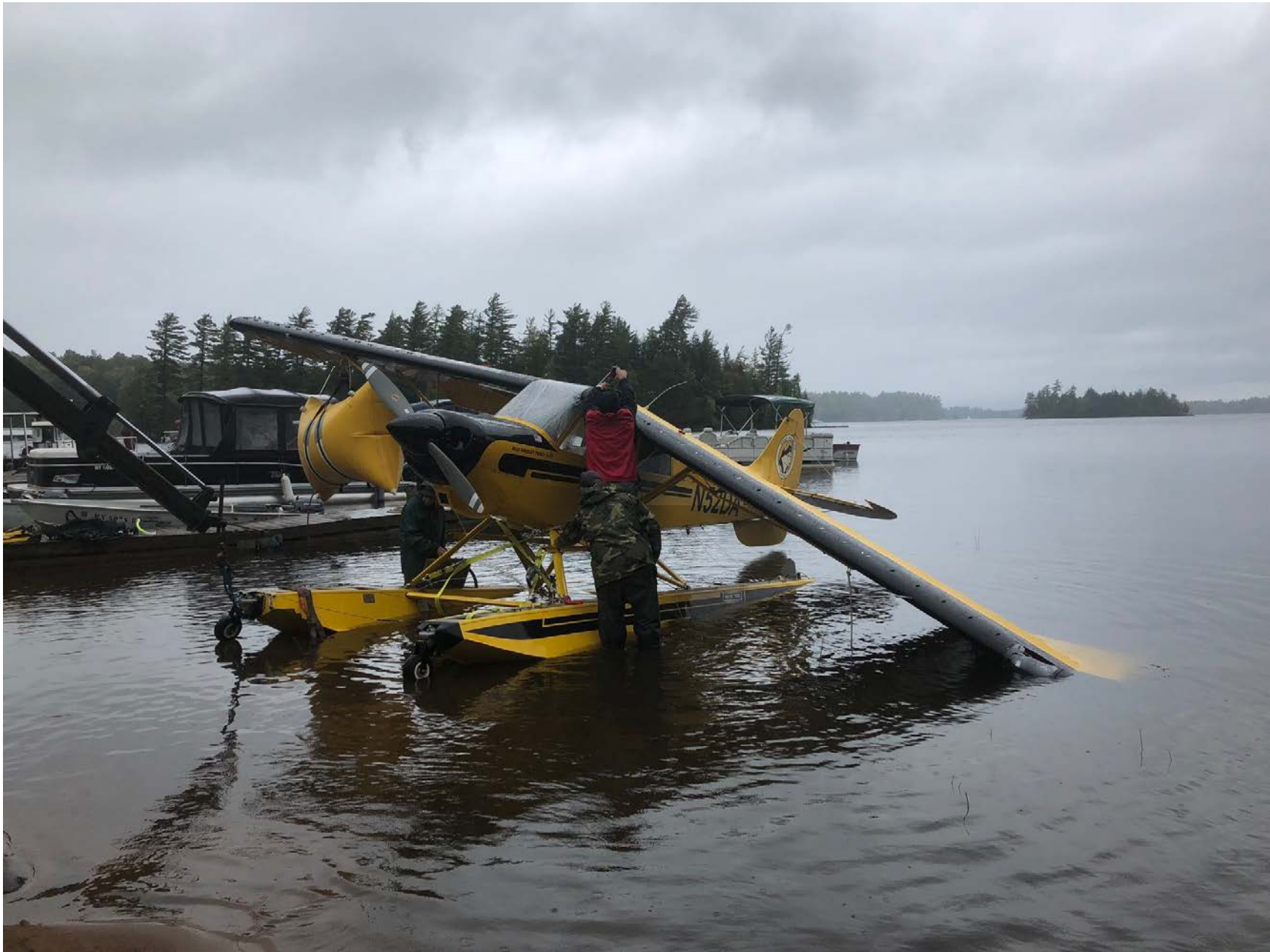
Photo 1 – View of damaged left wing lift strut (Photo courtesy of the pilot)
