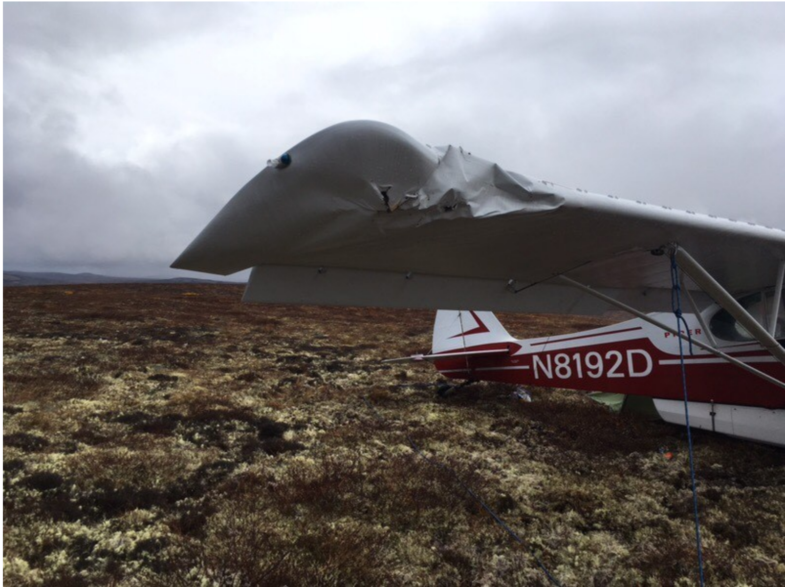
Photo 2 – View of damaged right wing (Photo courtesy of the pilot)
