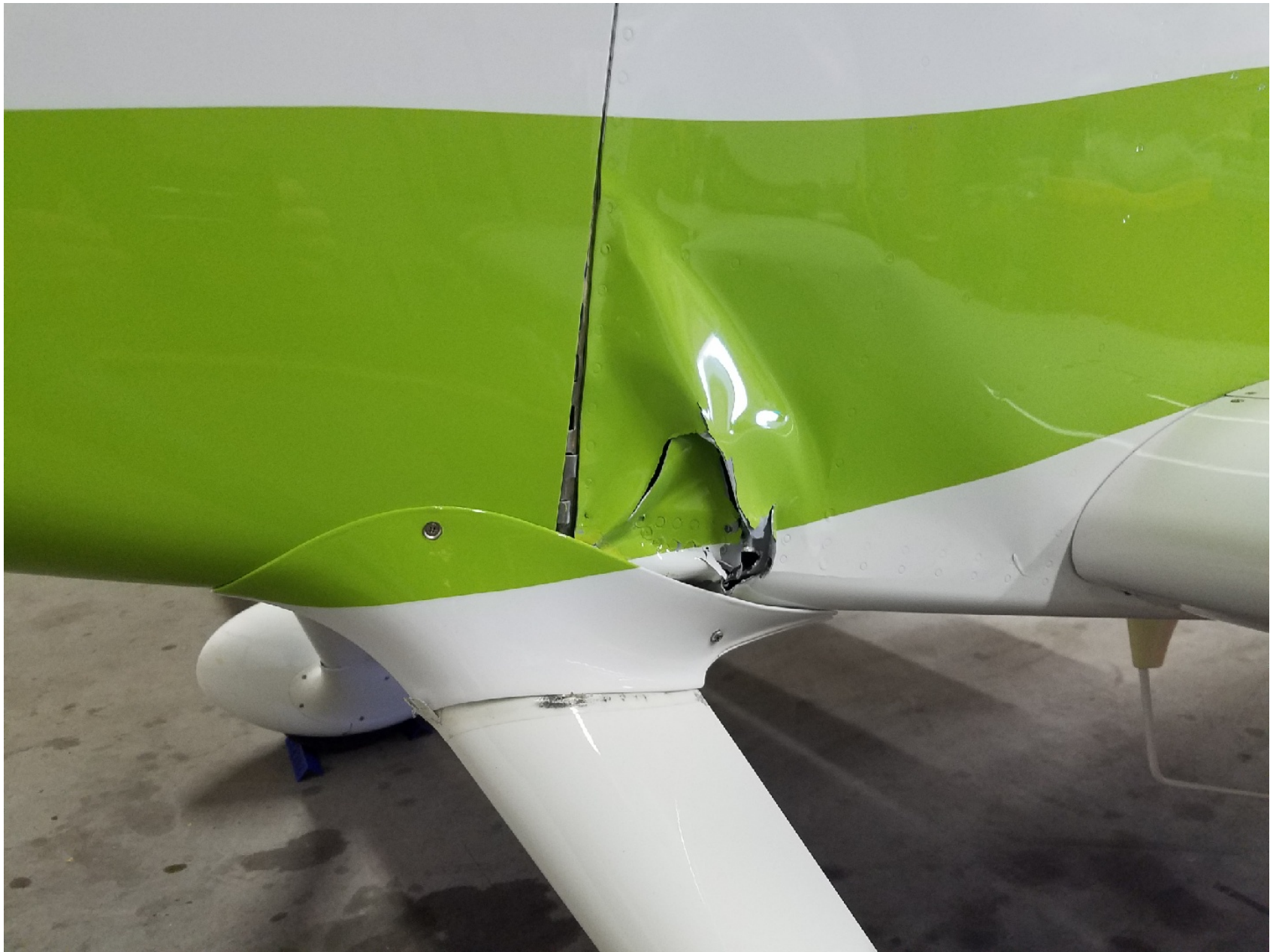
Photo 1 – View of damage to the landing gear attachment points (Courtesy of FAA)
