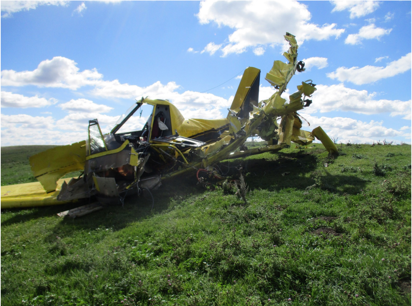
Photo 2 – View of damaged wings, fuselage, and empennage (Photo courtesy of the FAA)
