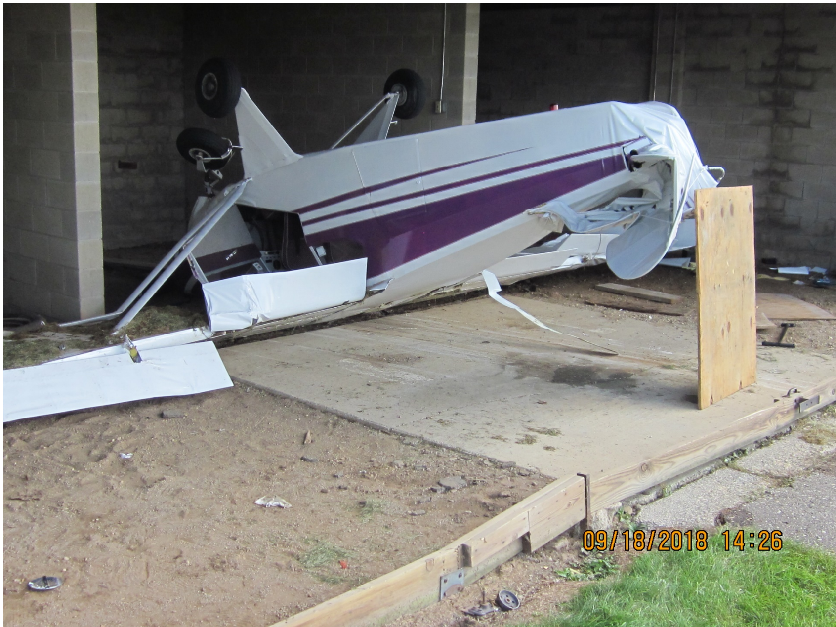
Photo 1 – View of inverted airplane and wing and empennage damage (Photo courtesy of the FAA)
