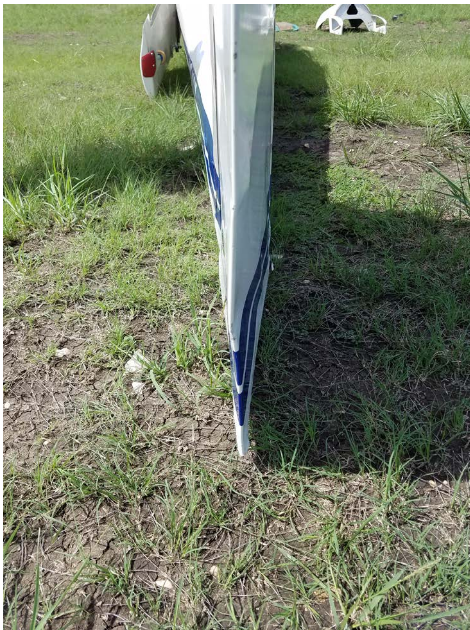
Photo 2 – View of damage to rudder (Courtesy of FAA)
