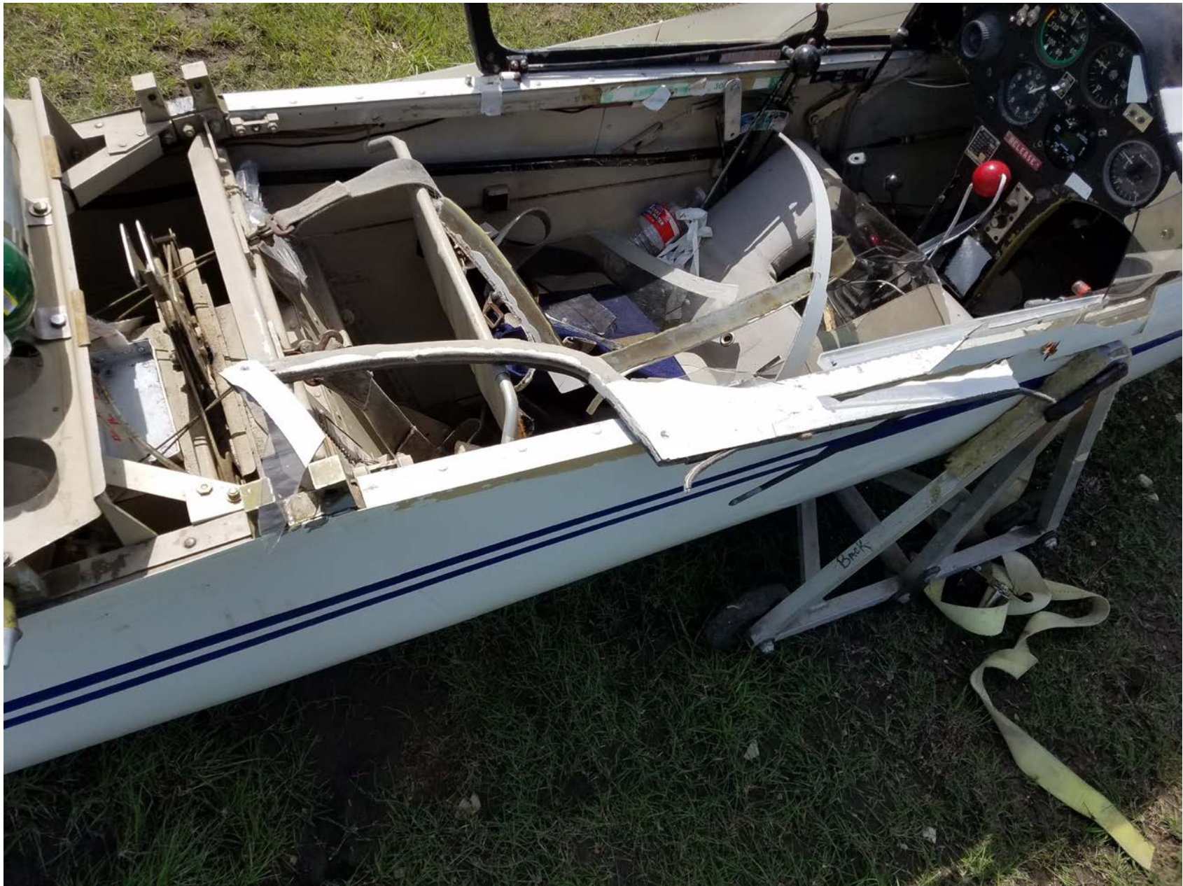
Photo 1 – View of damage to the canopy (Courtesy of FAA)
