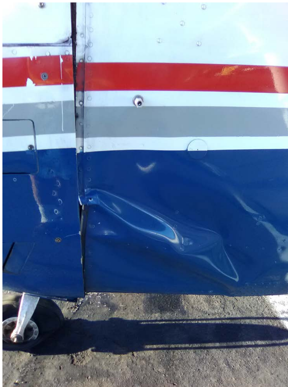
Photo 2 - View of damage to left, lower fuselage aft of engine firewall (courtesy of the FAA)
