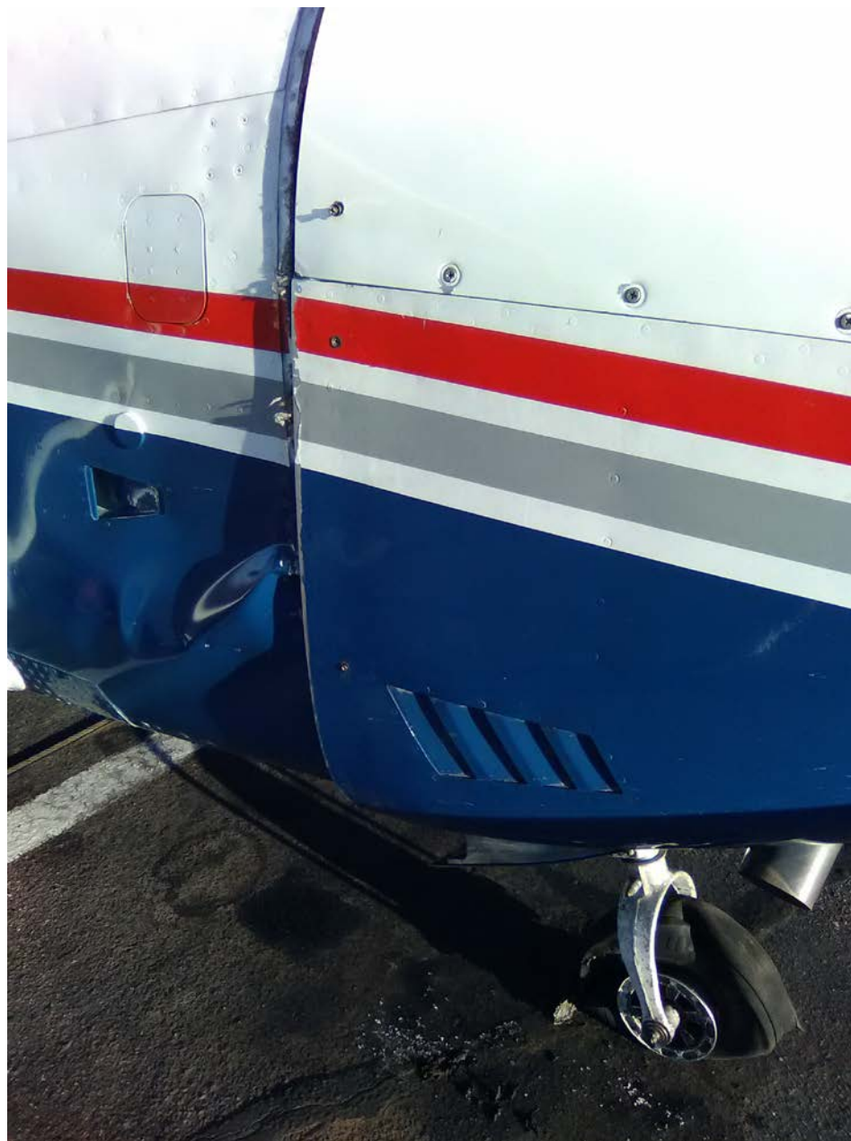
Photo 1 – View of damage to right, lower fuselage aft of engine firewall (courtesy of the FAA)
