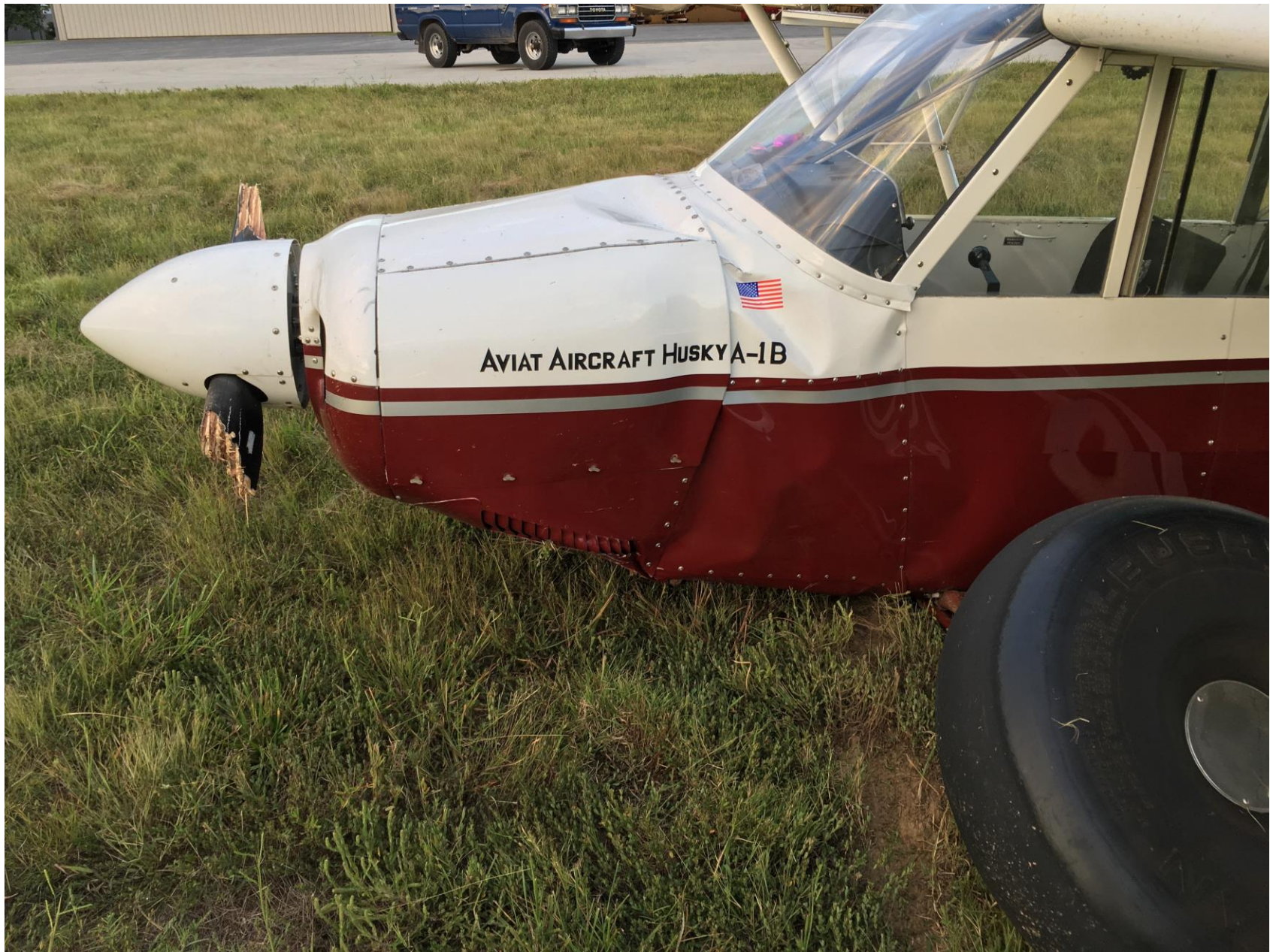
Photo 1 – View of damaged forward fuselage (Photo courtesy of the FAA)
