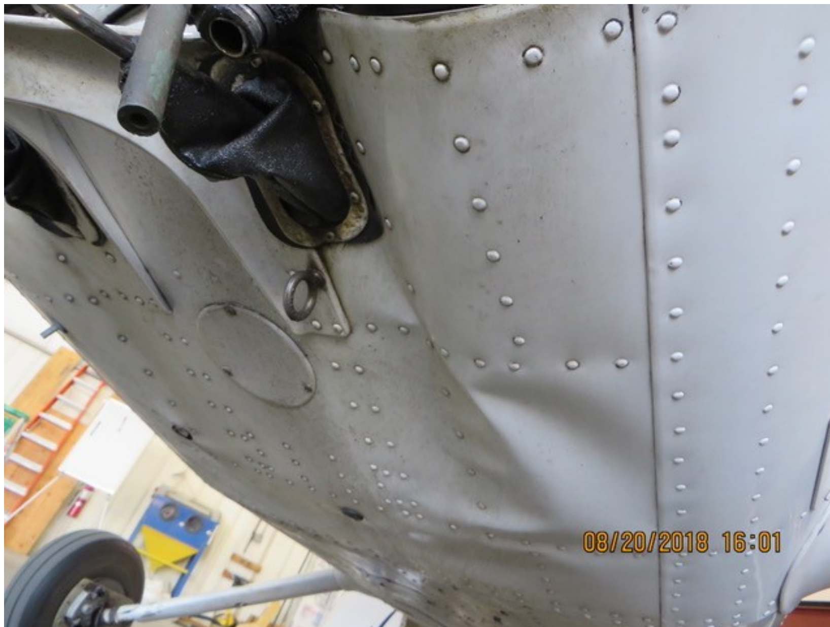
Photo 2 – View of damaged fuselage (Photo courtesy of the FAA)
