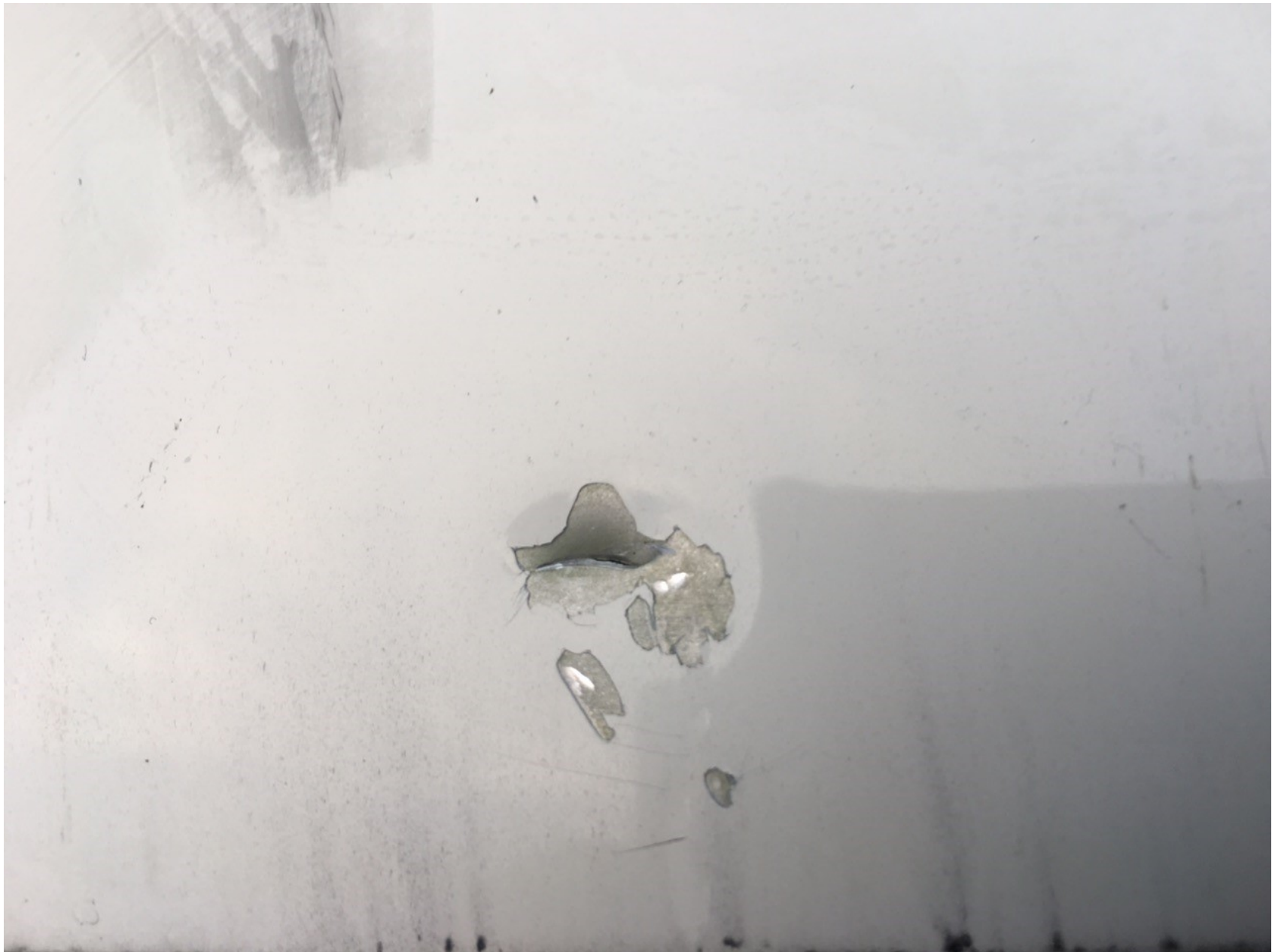
Photo 1 – Damage to main rotor blade (photo courtesy of FAA)
