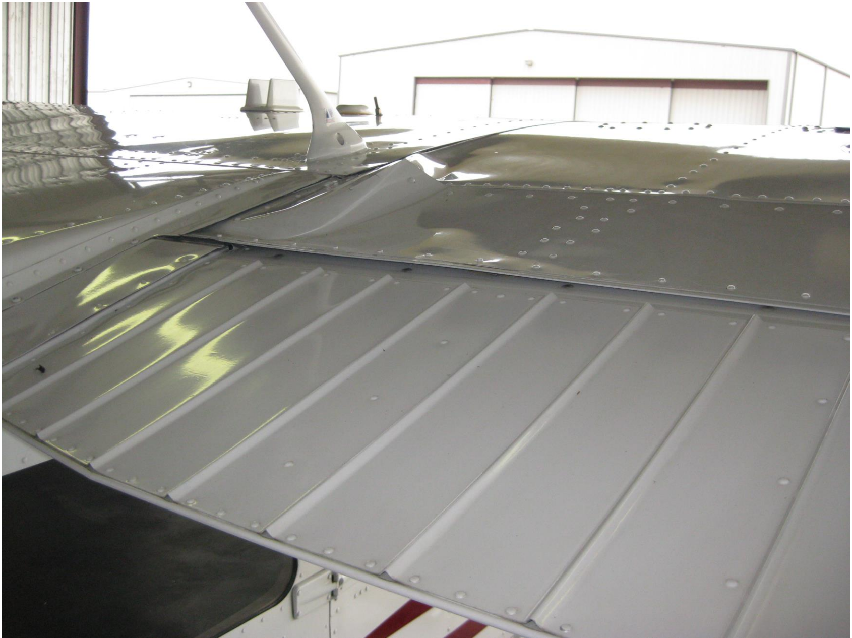
Photo 1 – View of right wing damage (Photo courtesy of the FAA)
