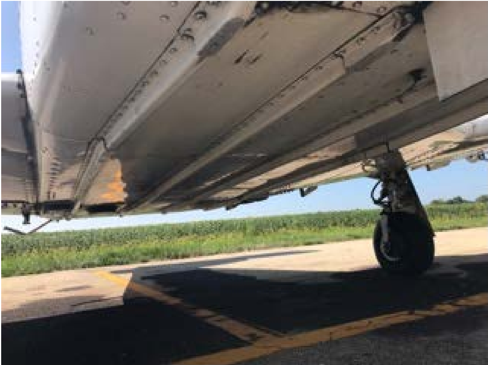
Photo 2 – View of damaged belly of fuselage (courtesy of the FAA)
