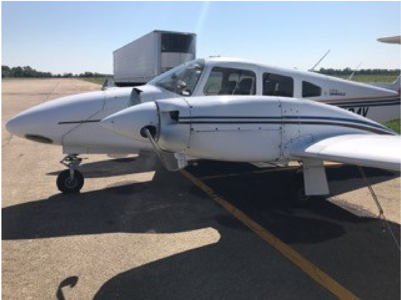
Photo 1 – View of damage to left and right-side propellers (courtesy of the FAA)
