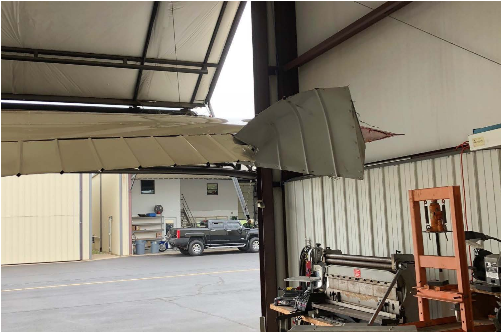
Photo 2 – View of damaged right aileron (Photo courtesy of the FAA)
