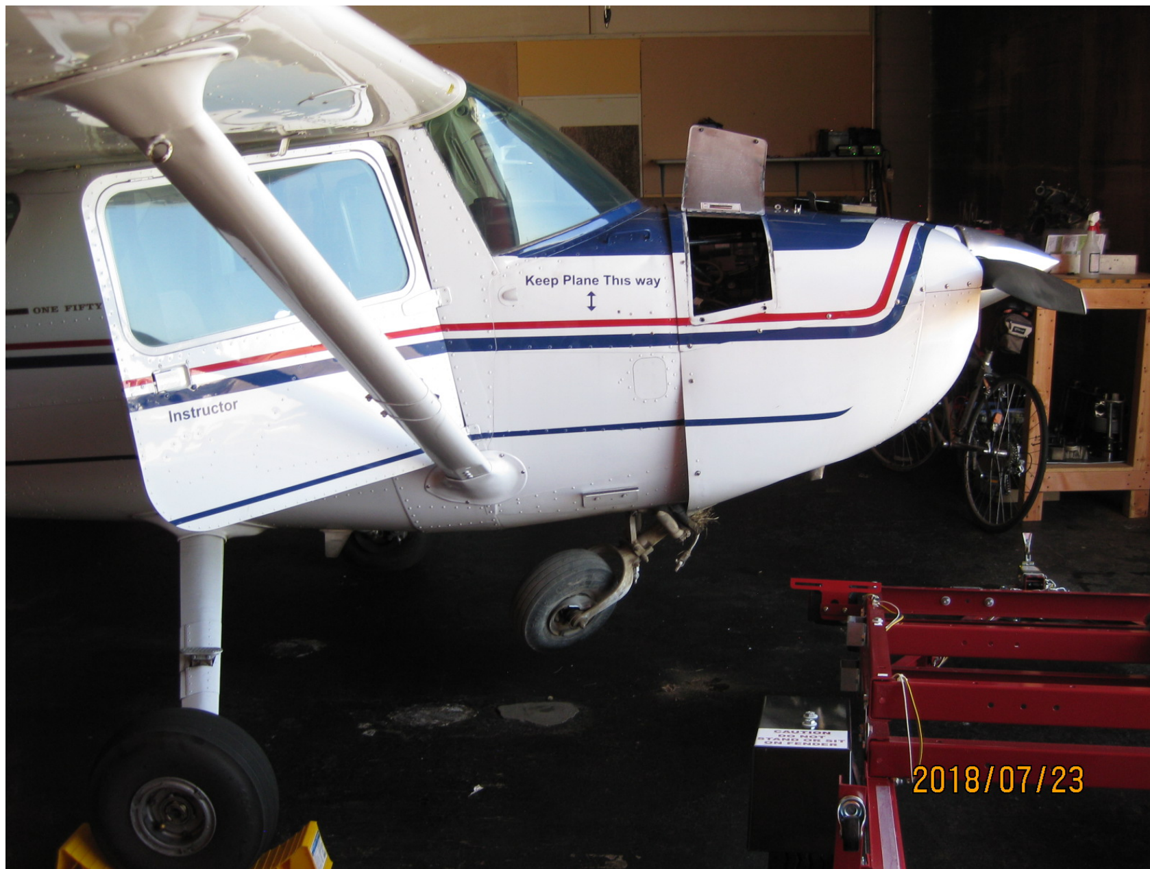
Photo 2 – View of propeller and damaged nose landing gear (courtesy of the FAA)
