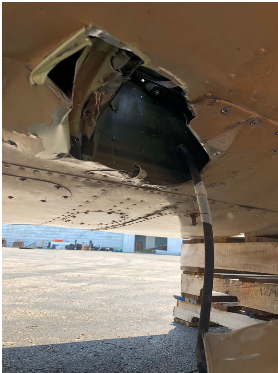
Photo 2 – View of damage to the right wing rib (Courtesy of FAA)
