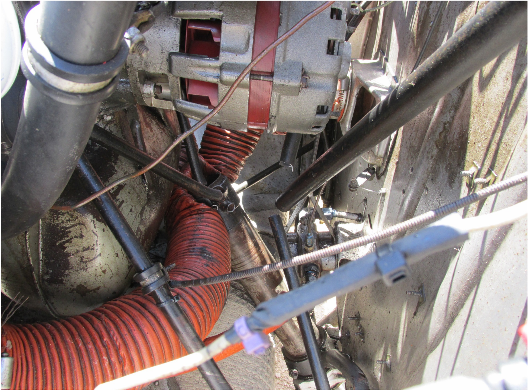
Photo 1 – View of damaged engine mount (Photo courtesy of the claims adjuster)
