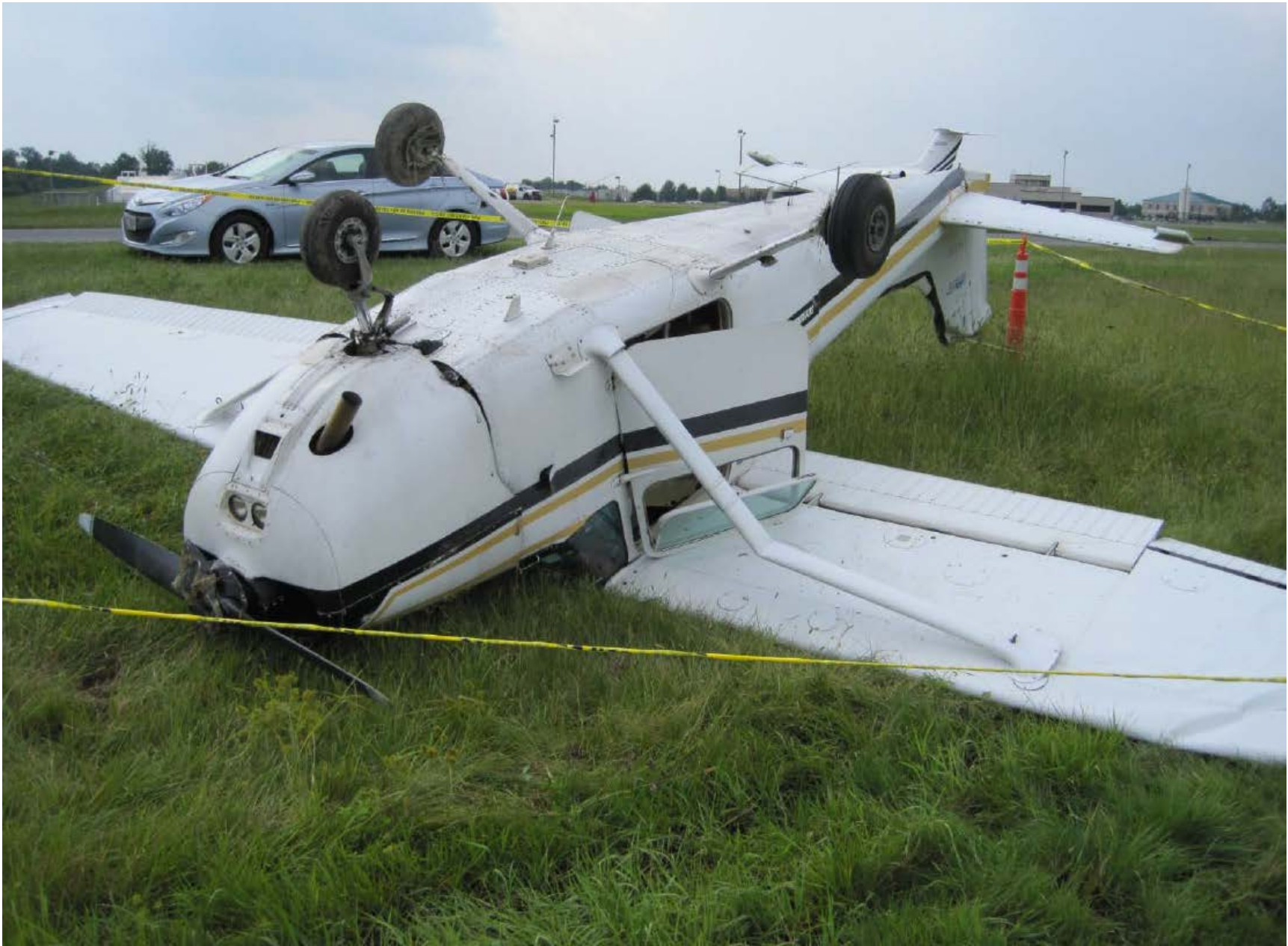
Photo 1 – View of damage to the right wing lift strut, vertical stabilizer and rudder (Courtesy of FAA)
