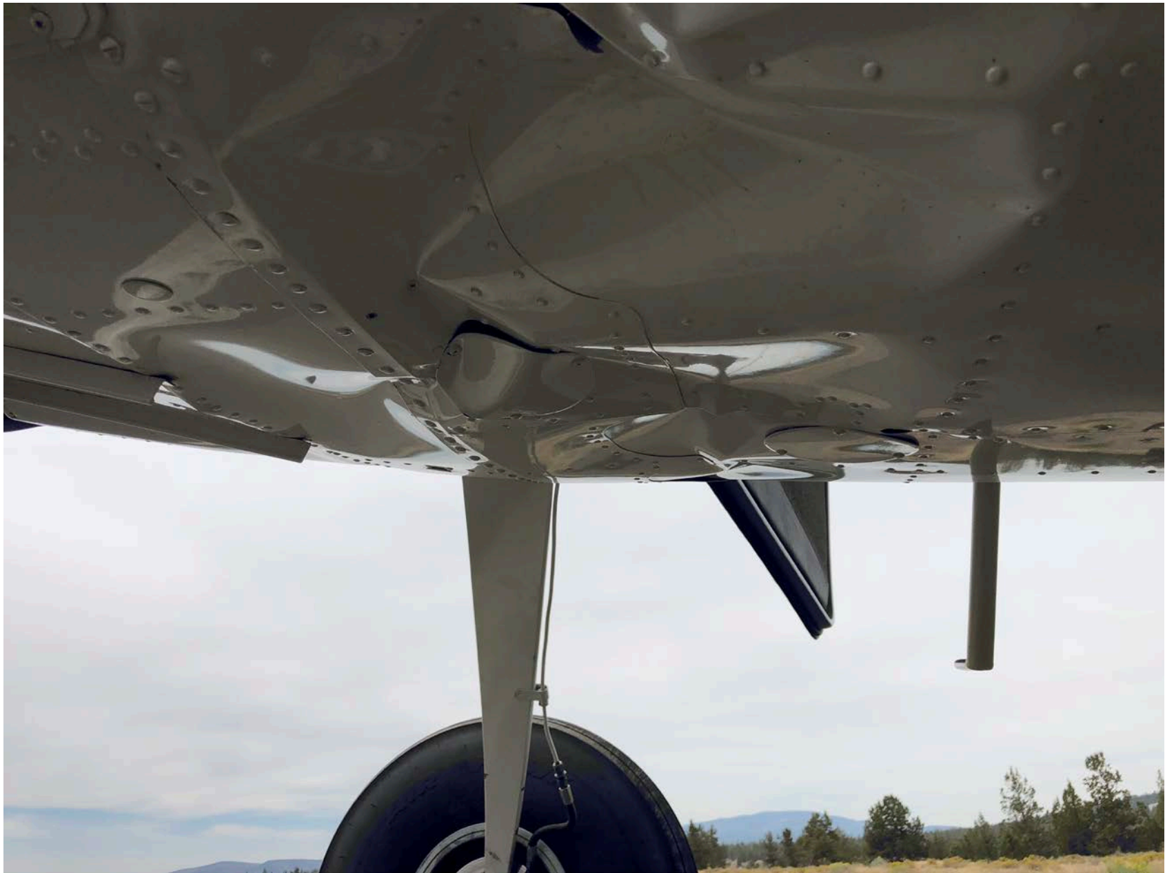
Photo 1 – View of damage to the forward lower fuselage bulkhead (Courtesy of FAA)
