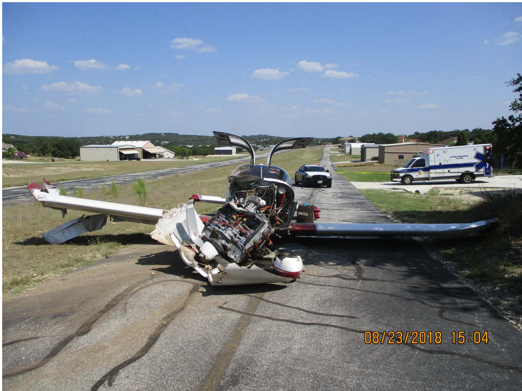
Photo 1 – View of damage to both wings, the right aileron, and the engine mounts (Courtesy of FAA)
