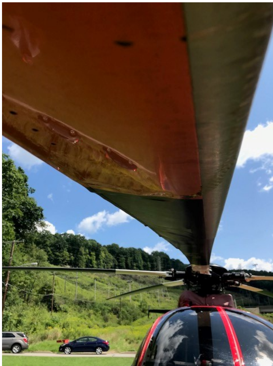
Photo – View of damaged main rotor blade (courtesy of the FAA)
