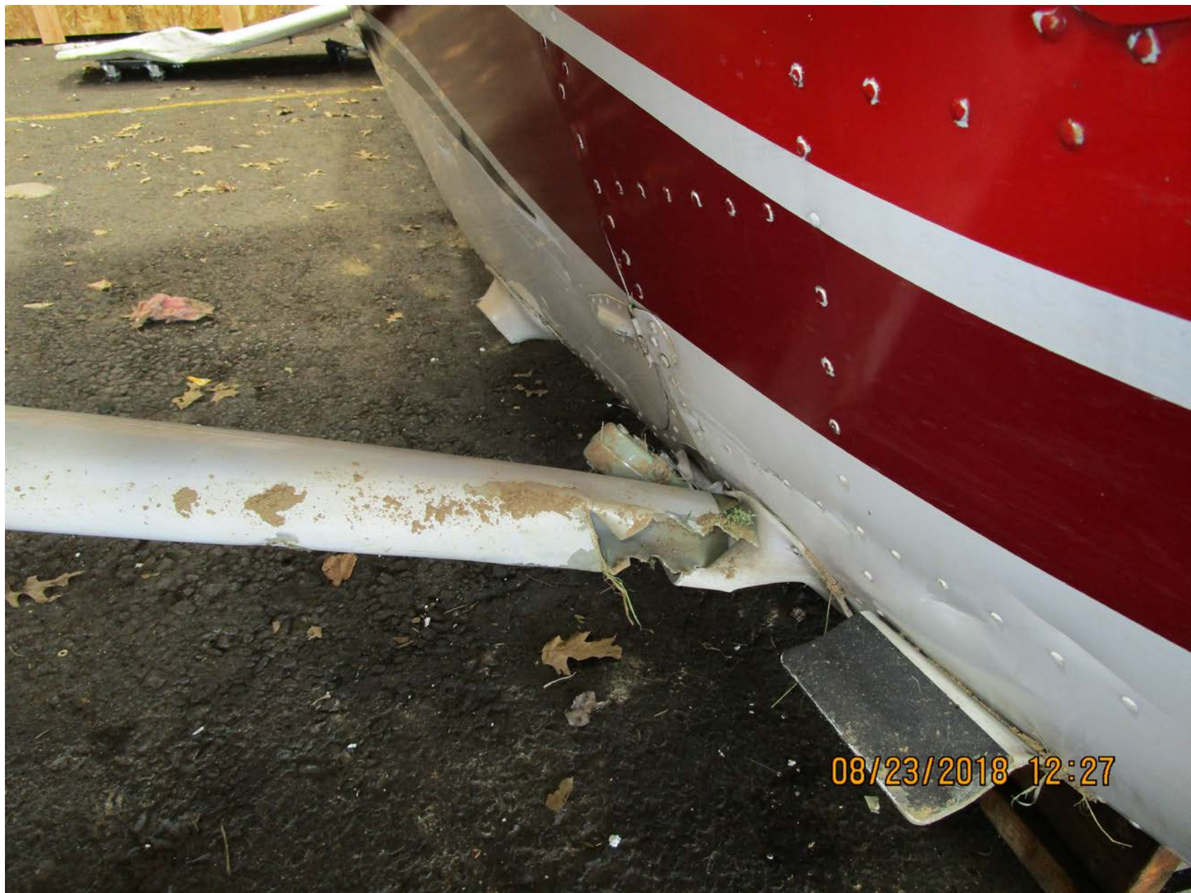
Photo 1 – View of damaged right wing lift strut and right horizontal stabilizer (courtesy of the FAA)
