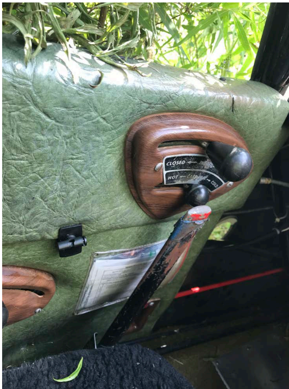
Photo 2 – View of carburetor heat position indicator (Courtesy of FAA)
