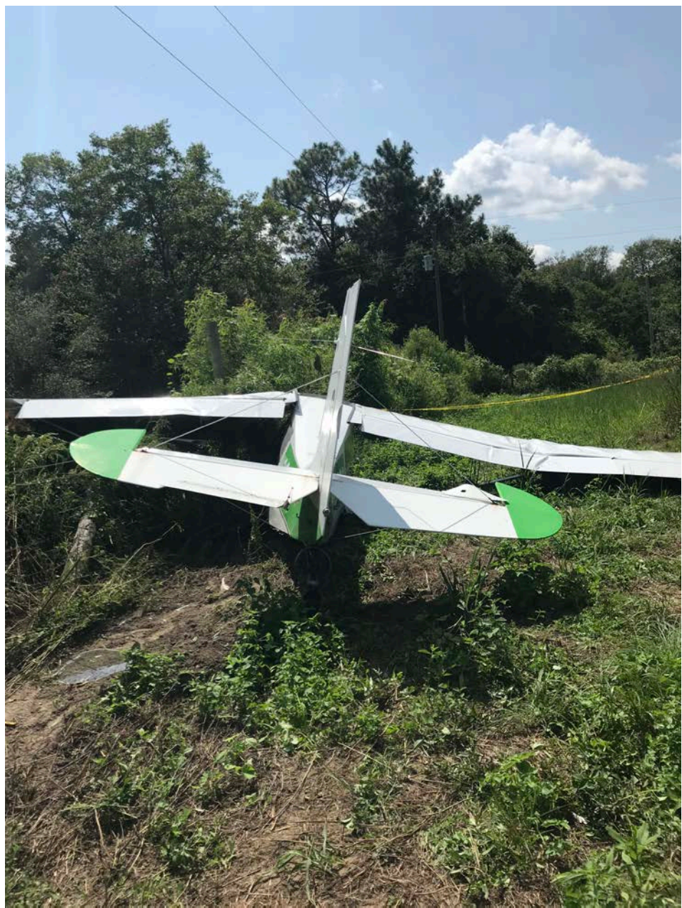
Photo 1 – View of damage to both wings (Courtesy of FAA)
