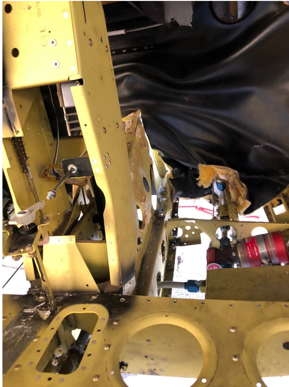
Photo 1 – View of damaged bulkhead and longeron (Courtesy of FAA)
