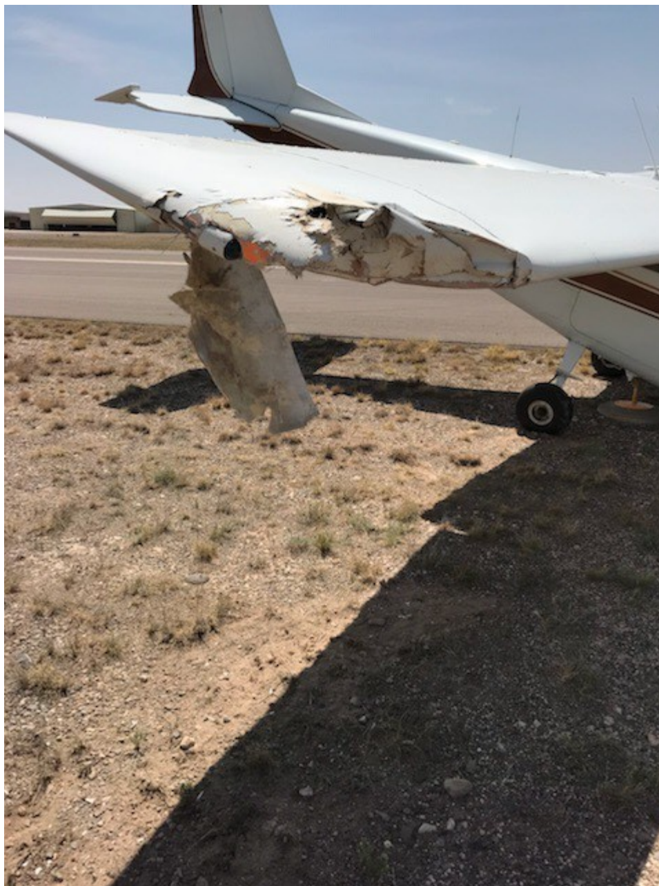
Photo 1 – View of damaged right wing (Photo courtesy of the FAA)
