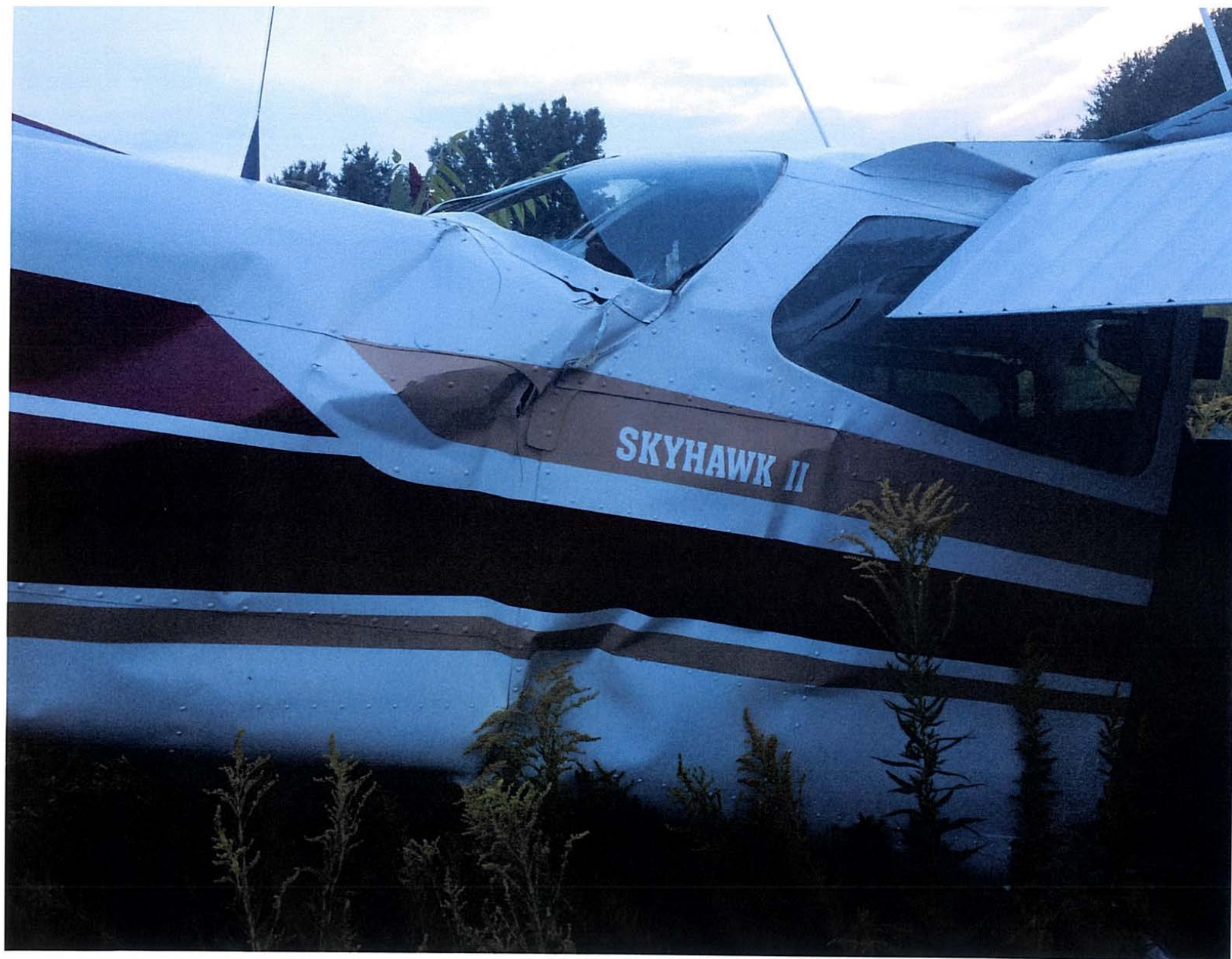
Photo 2 – View of damaged fuselage (Photo courtesy of local law enforcement)
