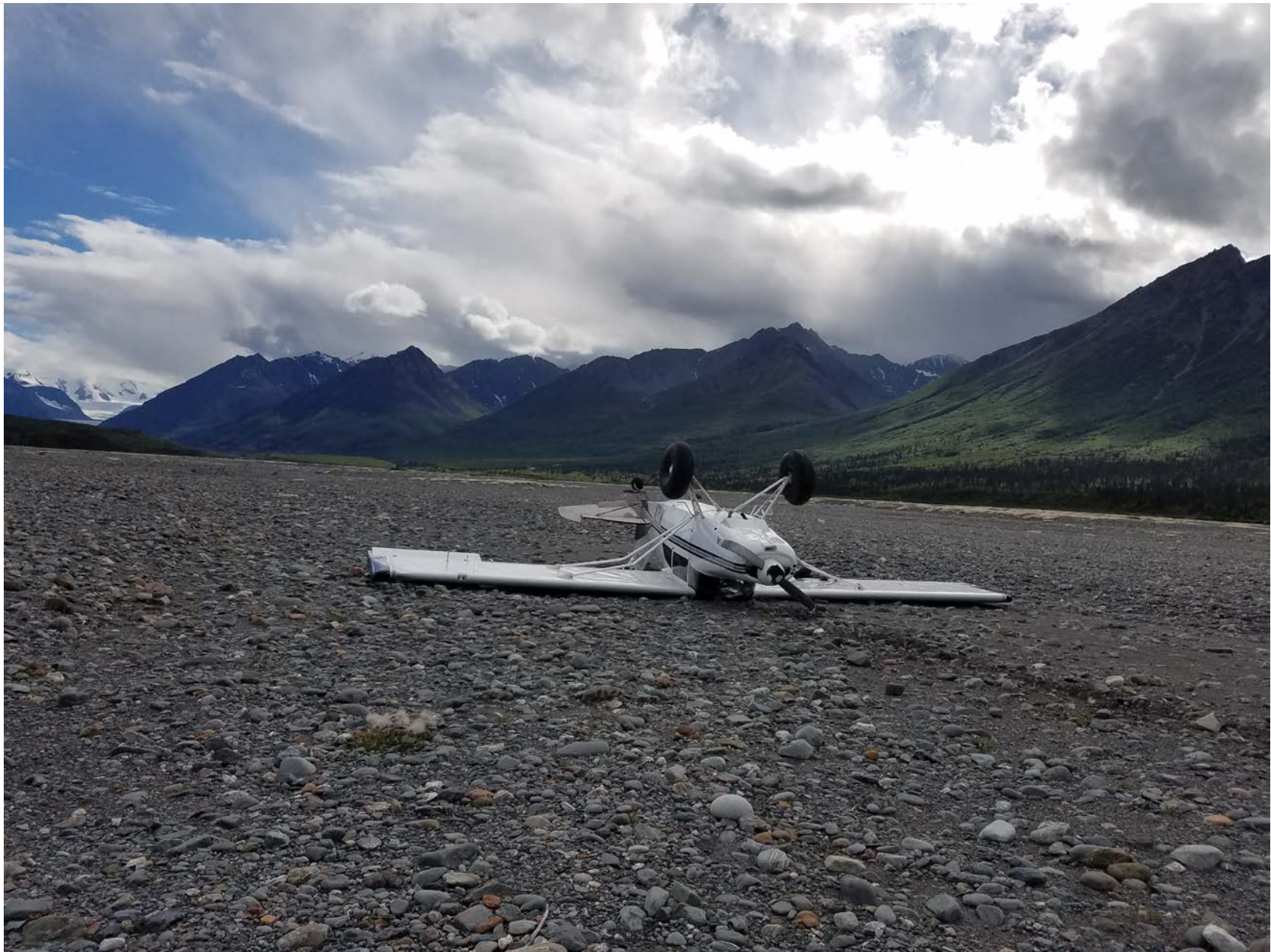
Photo – View of nosed over airplane with damaged left lift strut (courtesy of the pilot)
