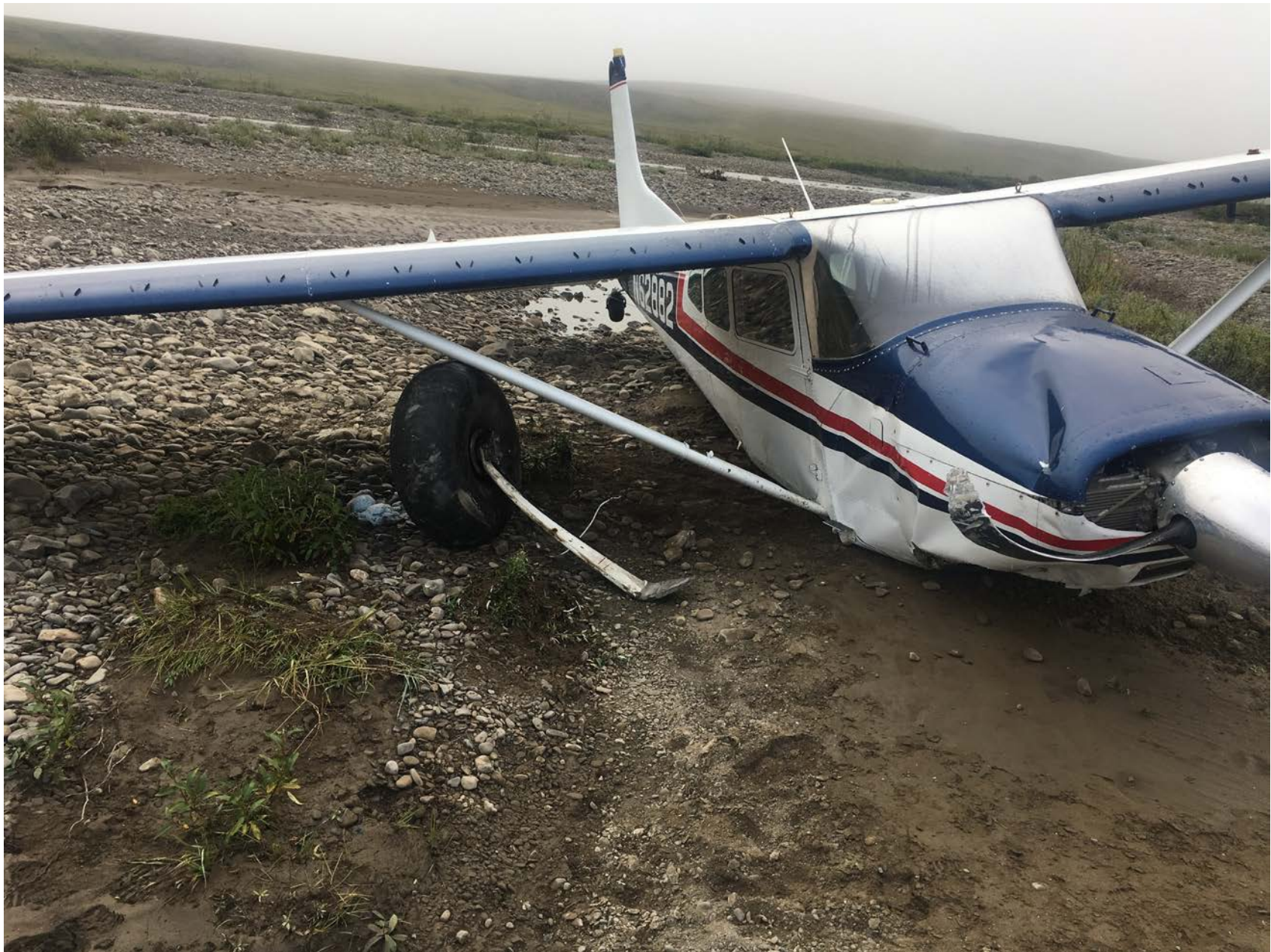
Photo 1 – View of damage to the forward right fuselage bulkhead assembly and stringer assembly (Courtesy of FAA)
