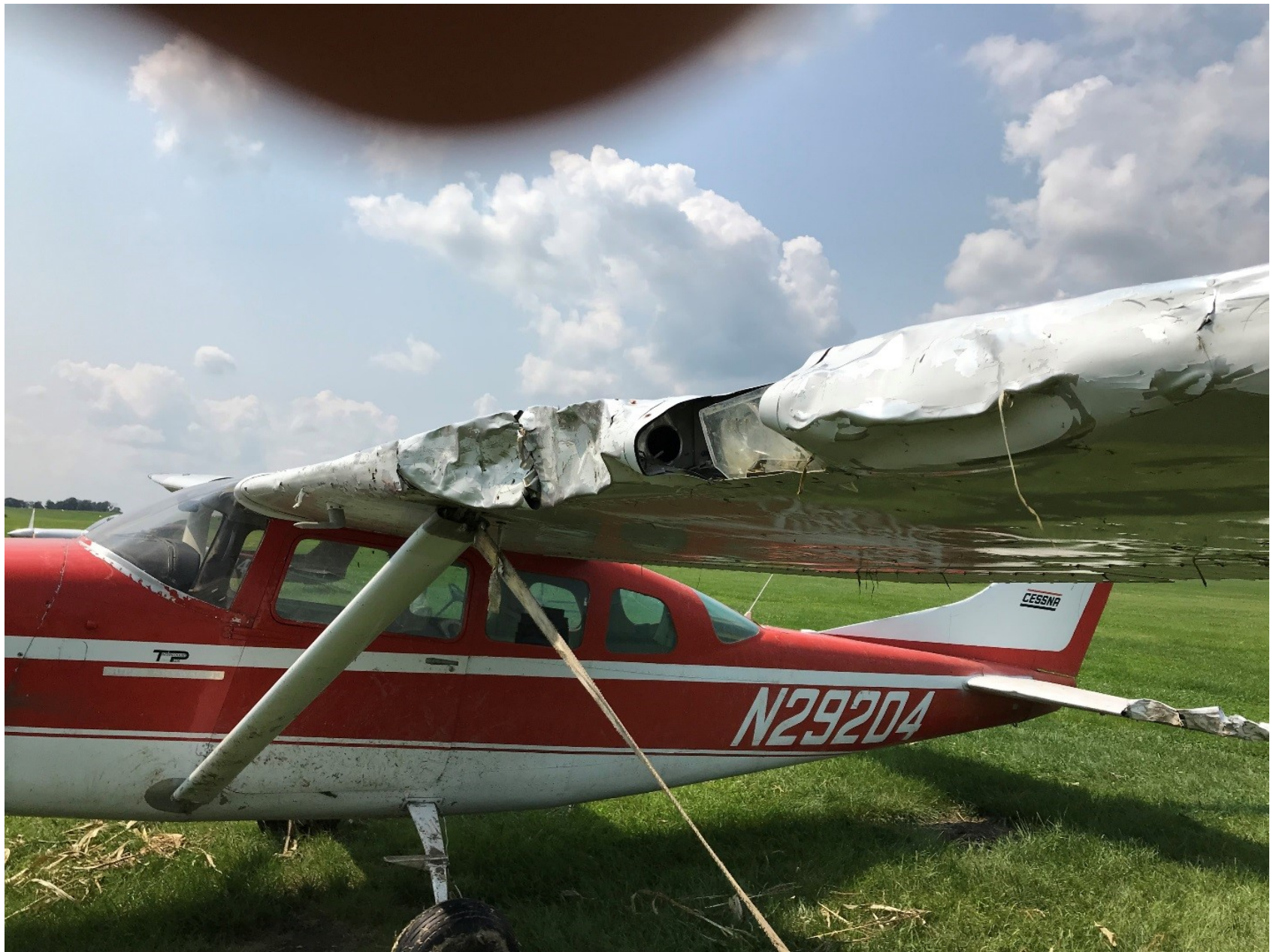
Photo – View of damaged left wing and horizontal stabilizer (courtesy of the FAA)
