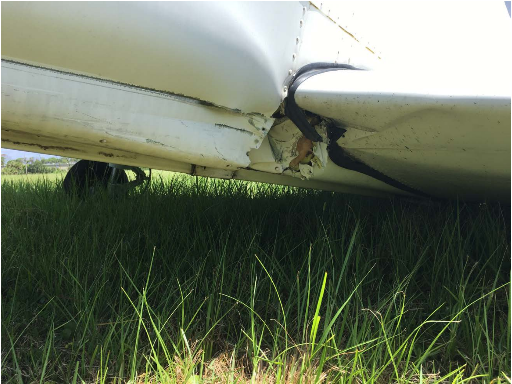
Photo 1 – View of damage to left wing and lower fuselage (courtesy of the FAA)
