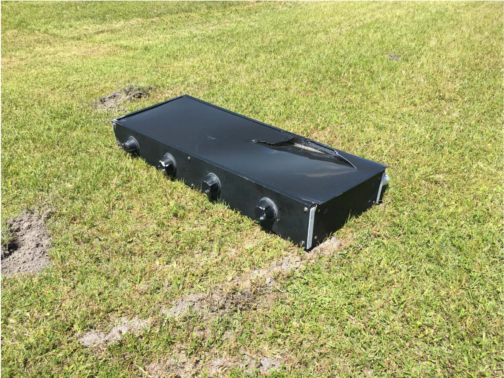
Photo 2 – View of damaged taxiway sign (courtesy of the FAA)
