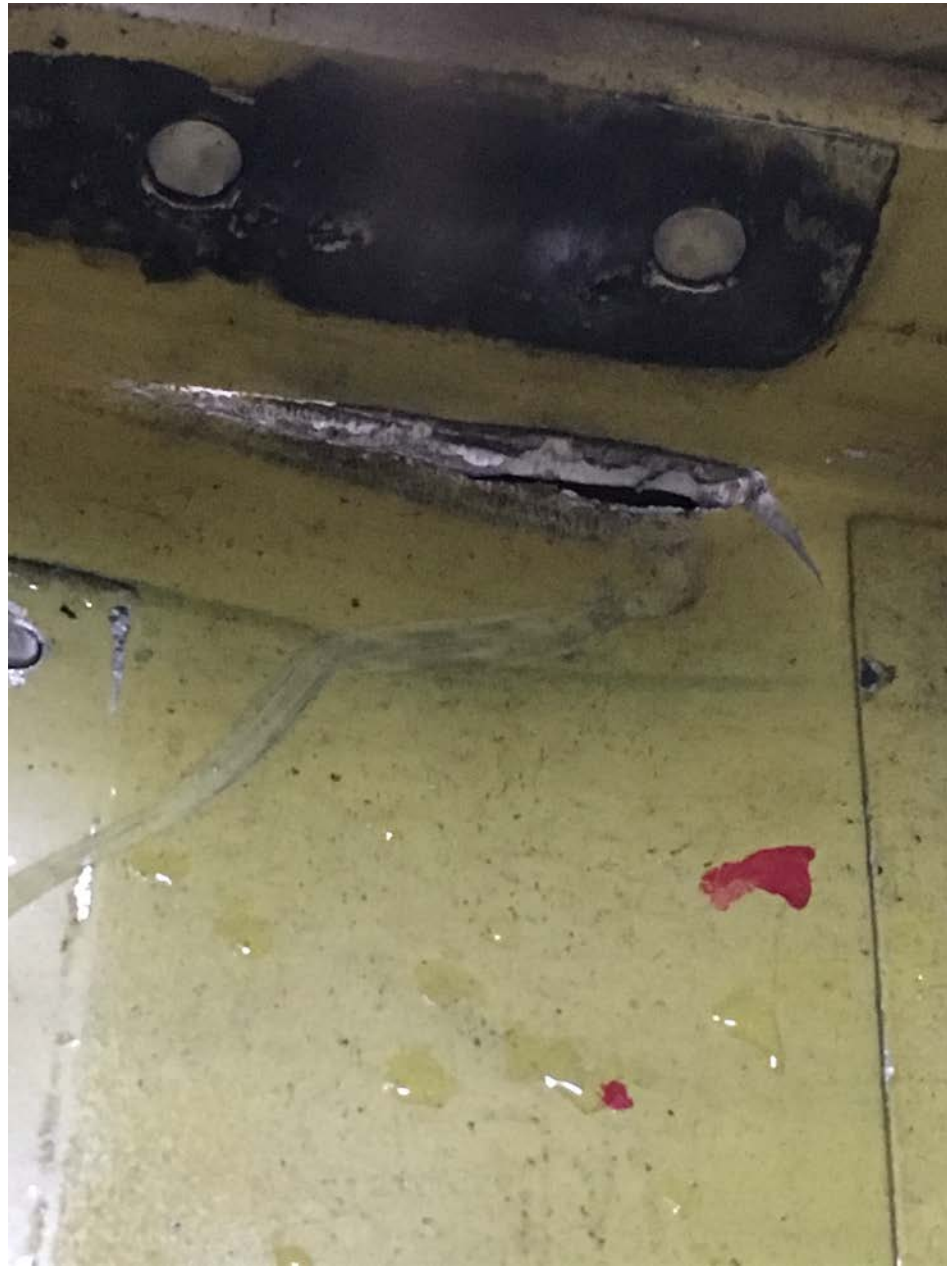
Photo 3 – View of damaged left-wing spar (courtesy of the FAA)
