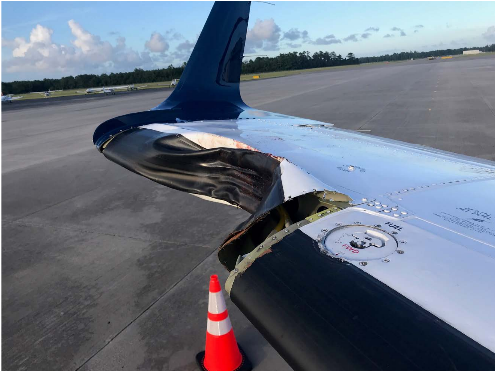
Photo 1 – View of damaged right wing leading edge (Photo courtesy of the operator)
