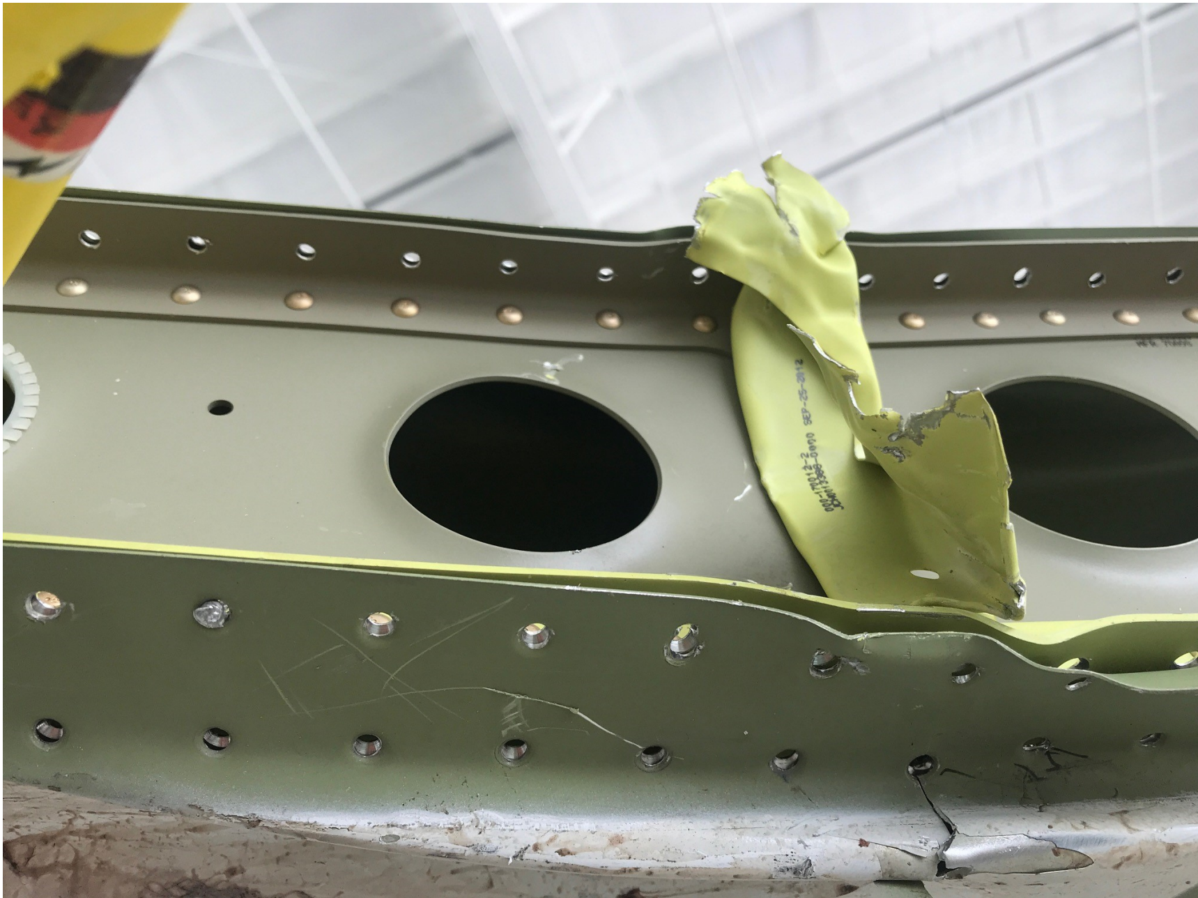
Photo 2 – View of damaged spar (Photo courtesy of the operator)
